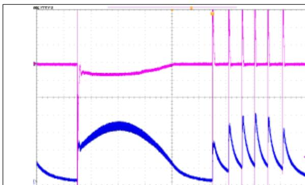
**Figure 7. TRIAC Current and Input Rectified Voltage Without RC-Damped Circuit**
