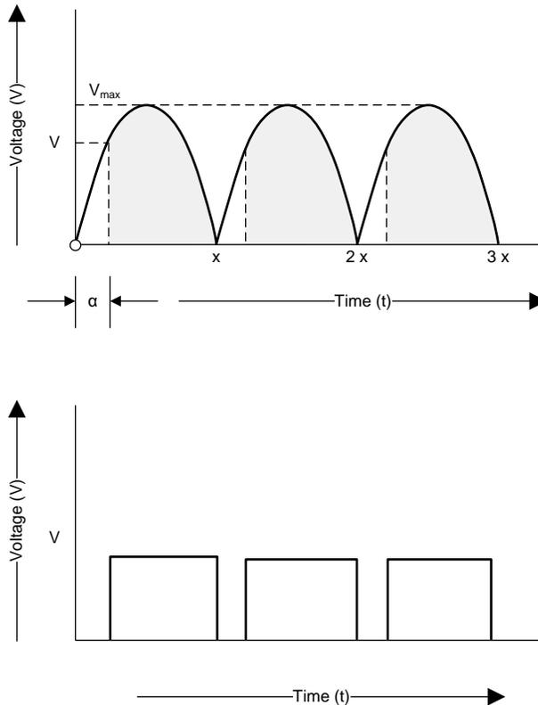
Figure 6. PWM Signal at Emitter of Optocoupler
