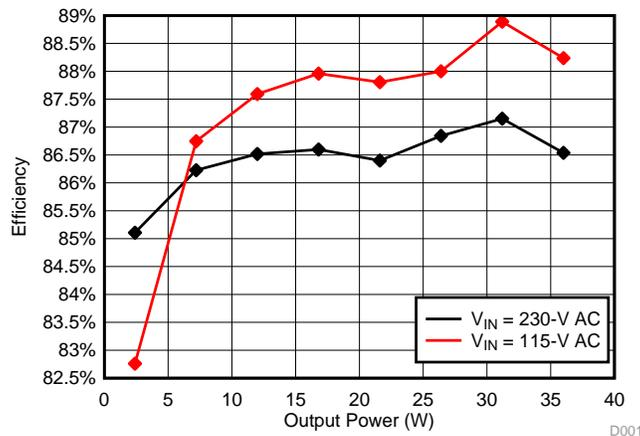
**Figure 9. Efficiency versus Output Power**
