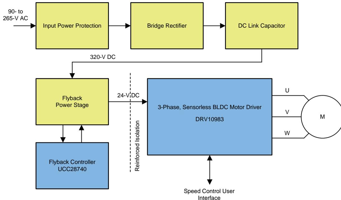
Figure 1. TIDA-01417 System Block Diagram
