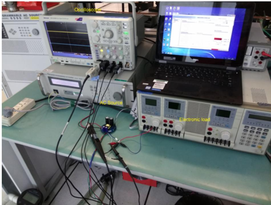
**Figure 5. Picture of Test Setup for Flyback Power**
