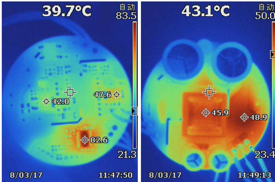
Figure 34. Temperatures for Motor Driver DRV10983
