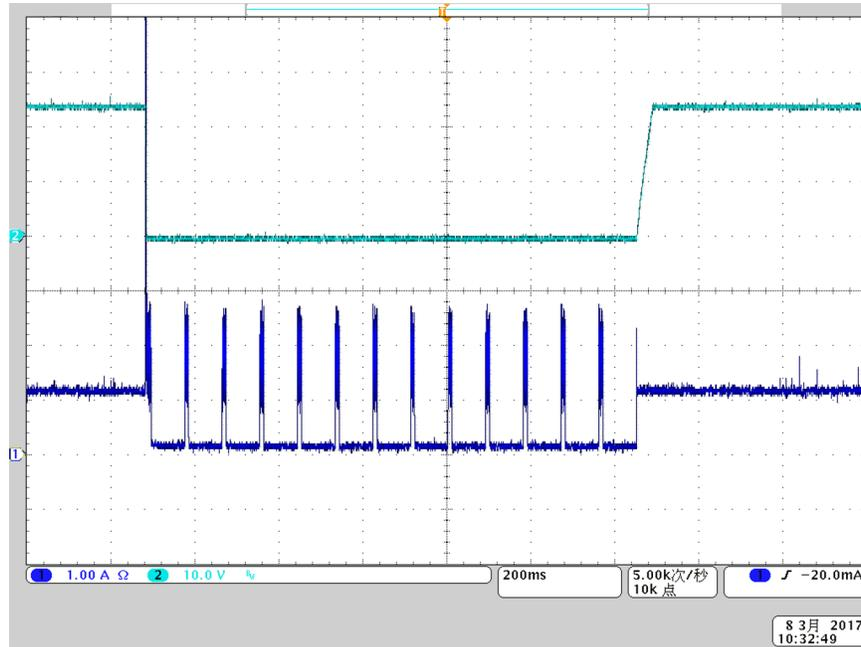
**Figure 23. Response During Short-Circuit and Auto-Recovery When Short is Removed**
