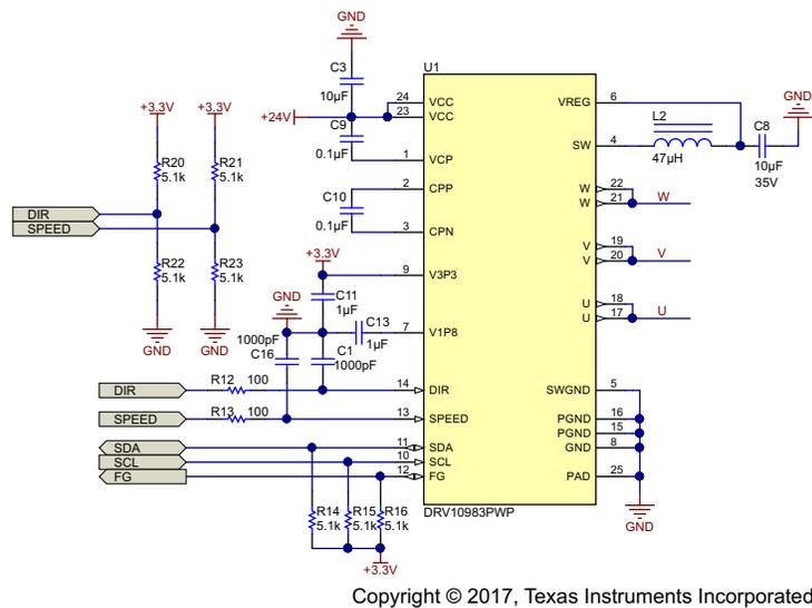
Figure 3. DRV10983 Motor Drive Schematic
