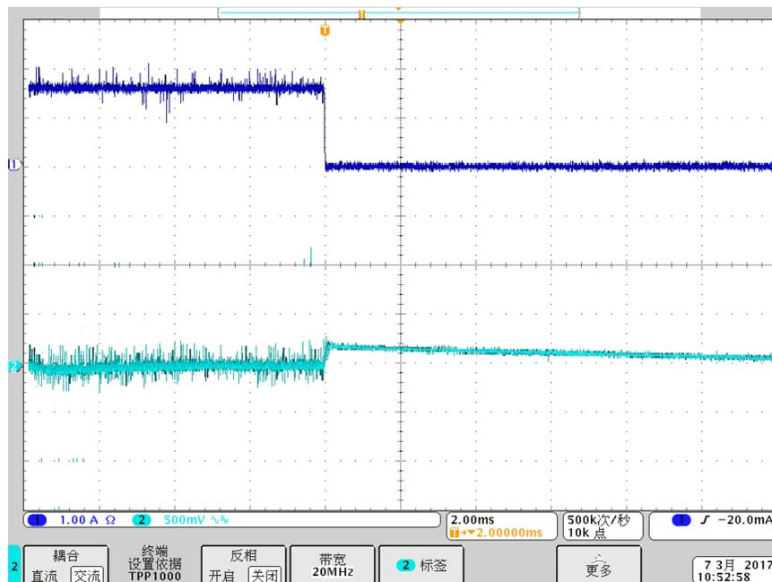
Figure 21. Output Voltage and Current Waveform, Load Transient From 1.5 to 0 A
