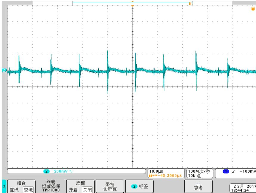
Figure 16. Output Voltage Ripple at  $V_{INAC} = 115\text{-V AC}$ , Full Load
