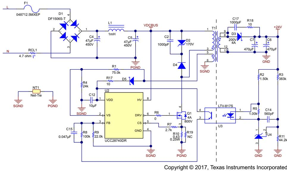
Figure 2. Flyback Power Supply Schematic
