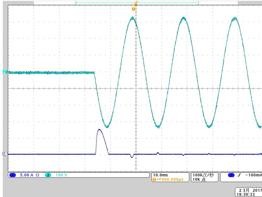
Figure 13. Input Inrush Current at 230-V AC
