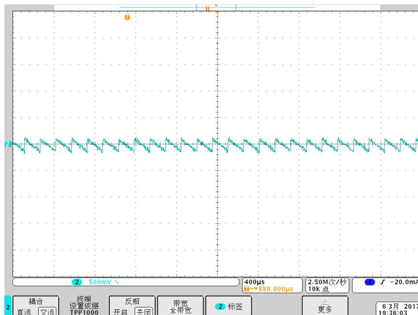
Figure 29. Ripple in 3.3-V Output From Step-Down Regulator of DRV10983
