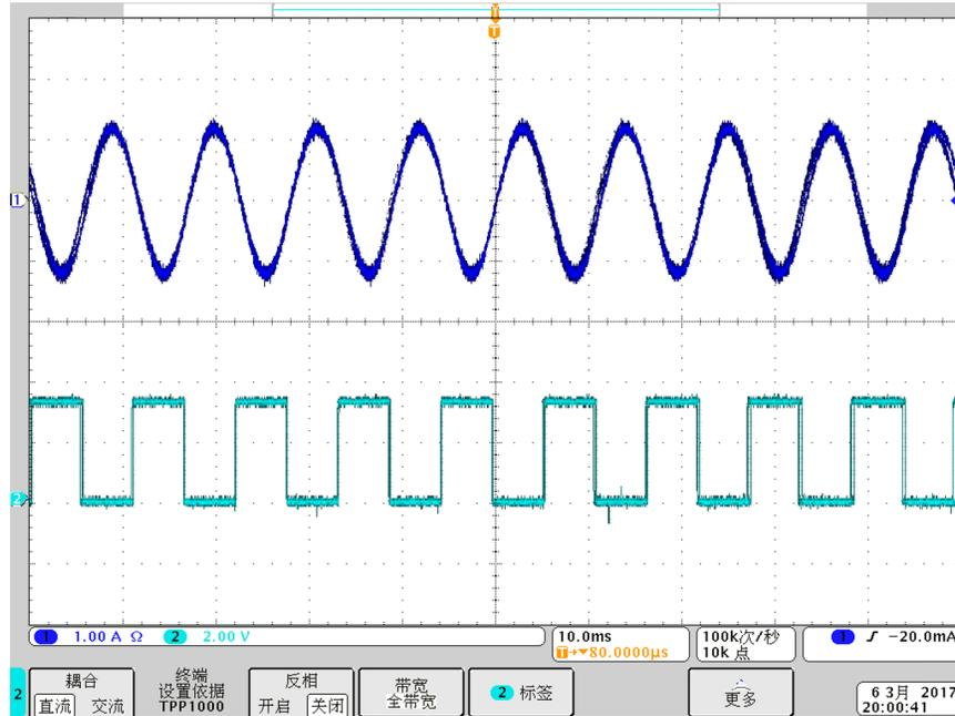
Figure 27. DRV10983 Speed Signal versus FG
