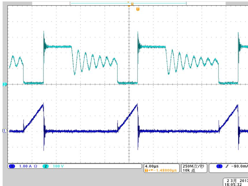
Figure 14. SW Node Waveform and MOSFET Current at  $V_{INAC} = 115\text{-V AC}$ , Full Load
