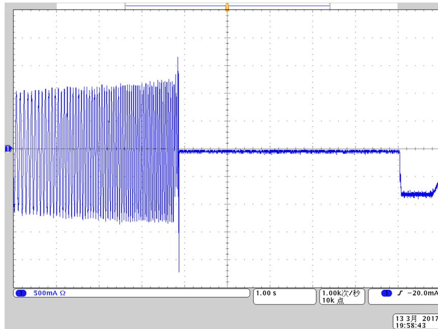
Figure 31. Winding Current Waveform During Rotor Lock
