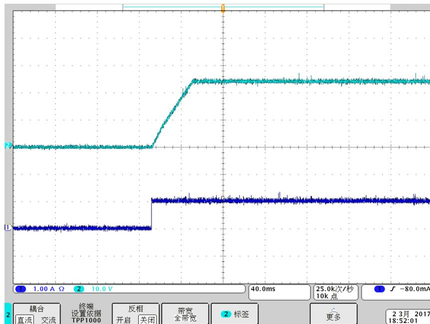
Figure 19. Output Turnon Waveform With CC Load of 1 A
