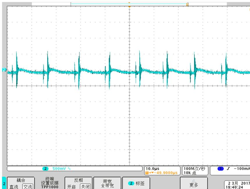
Figure 17. Output Voltage Ripple at  $V_{INAC} = 230\text{-V AC}$ , Full Load
