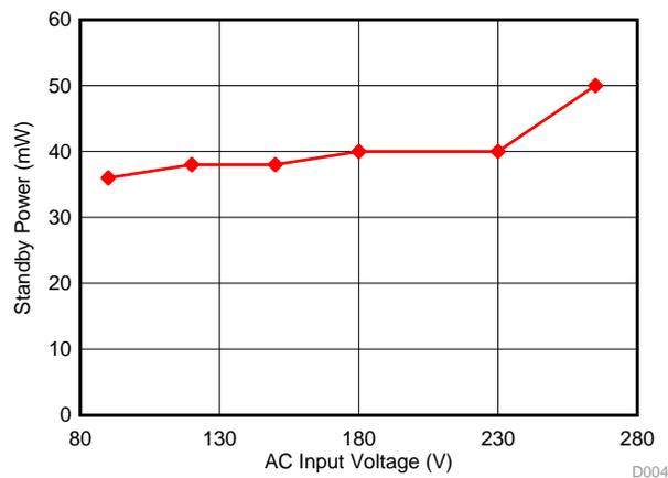
Figure 12. Standby Power With AC Input Variation
