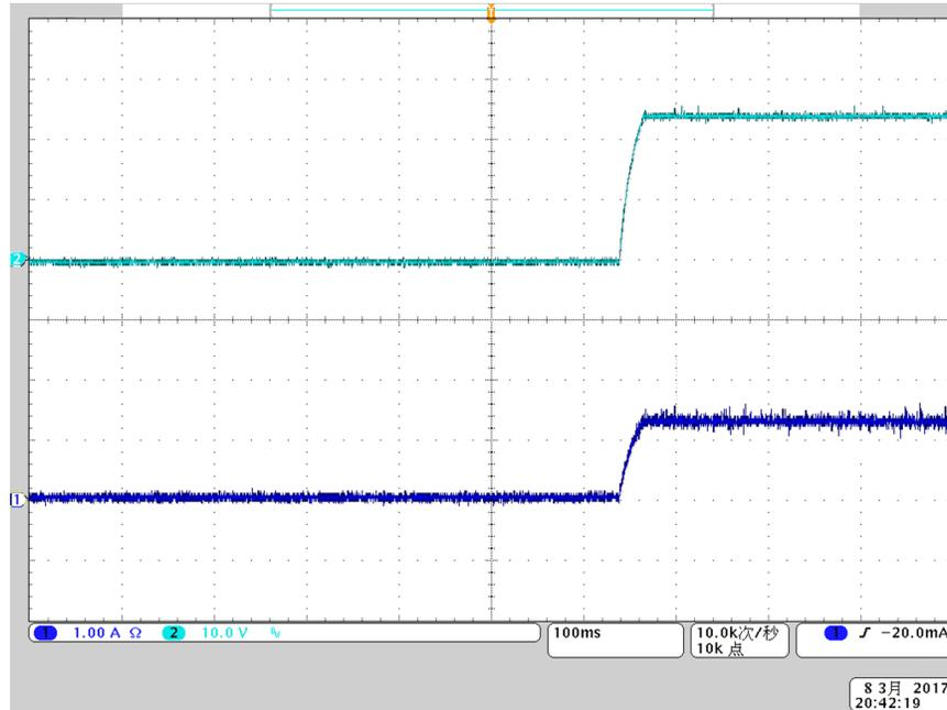
Figure 18. Output Turnon Waveform With Resistive Load of 21.5 Ω
