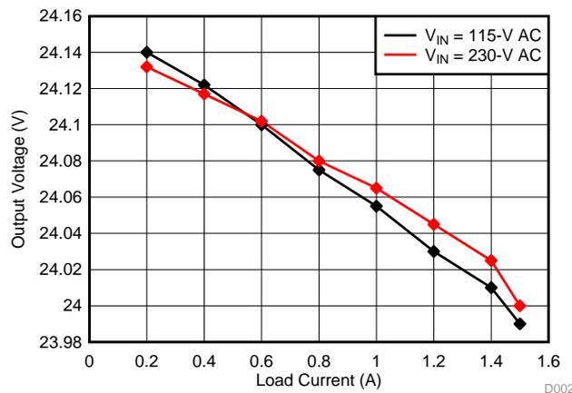
**Figure 10. Output Voltage Variation With Load Current**
