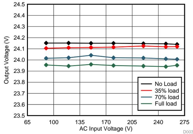
Figure 11. Load Regulation With Load Current
