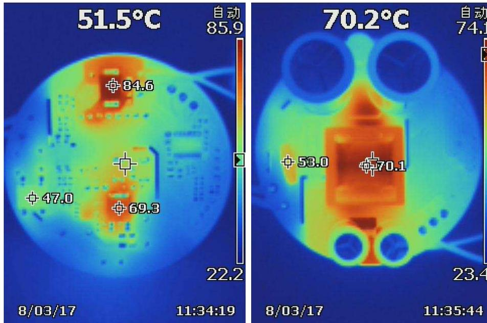
Figure 33. Temperatures at 230-V AC Input and 36-W Output
