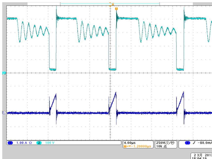
Figure 15. SW Node Waveform and MOSFET Current at  $V_{INAC} = 230\text{-V AC}$ , Full Load
