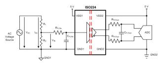
Figure 1. AC Voltage Sensing with the ISO224
