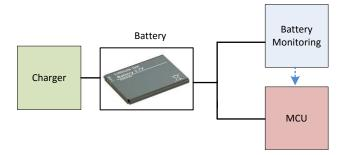
Figure 1. Mobile Phone Charging Stage
