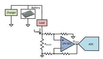
**Figure 3. Differential Amplifier Configuration**
