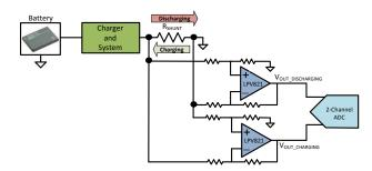
Figure 4. Bidirectional Current Sensing
