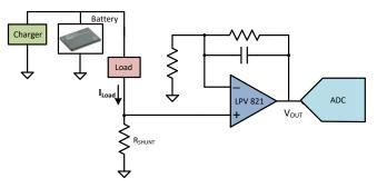
Figure 2. Single Ended Input Configuration
