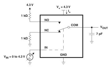
Figure A-3. Test Setup for Supply Currrent vs Control Input Voltage
