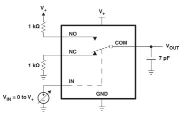
Figure A-2. Test Setup for Competitor Device ( $V_{OUT}$  vs  $V_{IN}$ )
