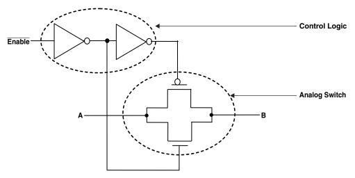
Figure 3. Internal Structure of a Typical Analog Switch
