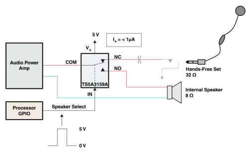
Figure 4. No Excess Current Consumption – Supply Voltage and Control Input Are at Same Voltage Level
