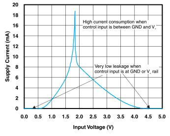
Figure 1. Supply Current vs. Control Input Voltage for the TS5A3159A (V<sub>+</sub> = 5 V)
