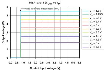
Figure 8. Control Input Threshold is Independent of V<sub>+</sub>
