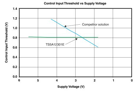
Figure 10. TS5A12301E Has a Constant Threshold Even as the Battery Discharges
