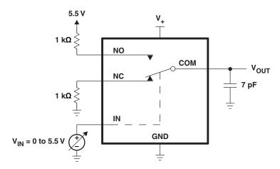
Figure A-1. Test Setup for TS5A12301E (V<sub>OUT</sub> vs V<sub>IN</sub>)
