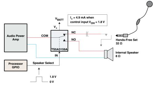
Figure 5. Excess Current Consumption – Control Input Is at Lower Voltage Than V<sub>+</sub>
