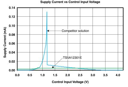
Figure 11. Comparison of Supply Current Between Competitor Solution and TS5A12301E
