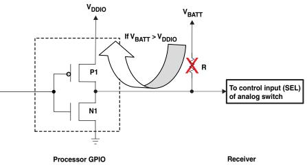
Figure 6. Drawbacks of Using a Pullup Resistor Directly From Processor GPIO to  $V_{\text{BATT}}$  for Up-Translation
