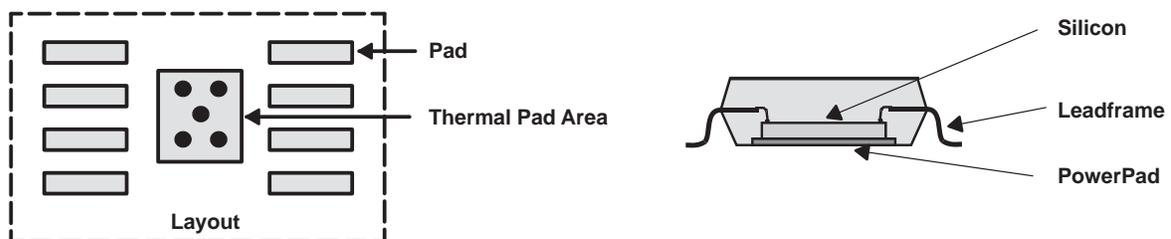
**Figure 6. PowerPAD™ Improves Heat Sinking**
