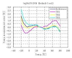
Figure 5. Plotted Temperature Readings from TI bq20z75 EVM Using Non-optimized Temperature Coefficients
