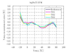
Figure 3. Plotted Temperature Readings from TI bq20z75 EVM with Optimized Coefficients
