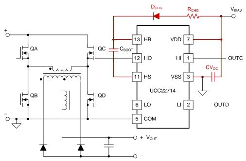
Figure 6. Simplified Gate Driver Schematic
