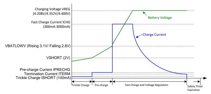
Figure 1. Battery Charging Profile
