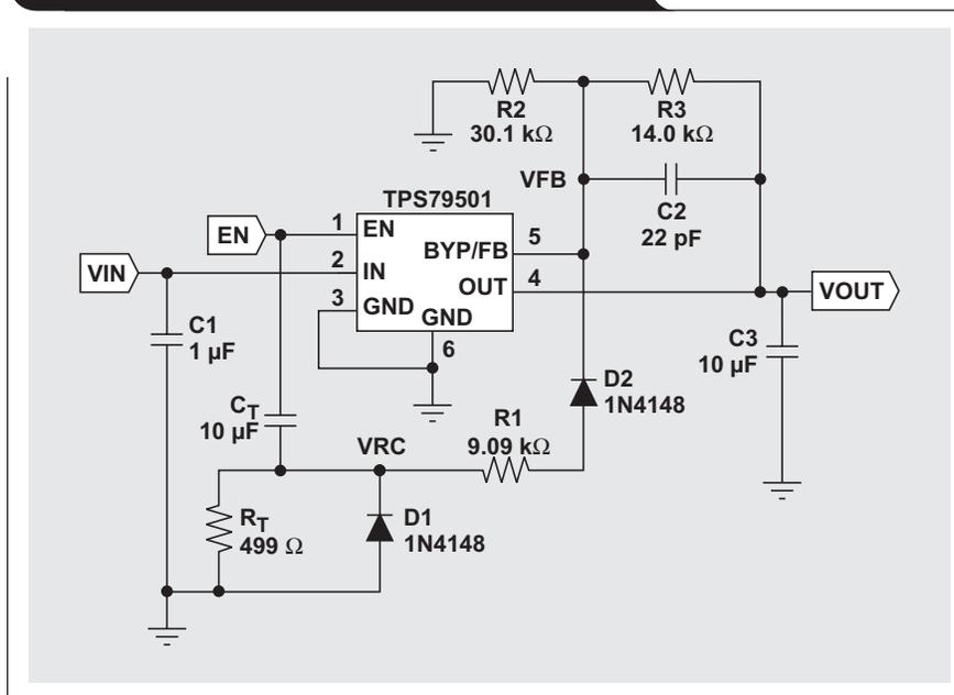
200 mV above the intended feedback voltage but less than a diode drop below  $V_{EN}$ . Capacitor  $C_T$  then discharges through  $R_T$  and, as the feedback voltage drops, the pass element slowly turns on and the output voltage slowly rises. Diode D2 keeps R1 and  $R_T$  out of the feedback-voltage divider and therefore prevents any degradation in output-voltage tolerance during normal operation. Diode D1 clamps node  $V_{RC}$  to a diode drop below ground when EN is taken low.
