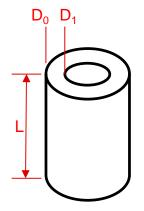
Figure 23. Conduction Through Via
