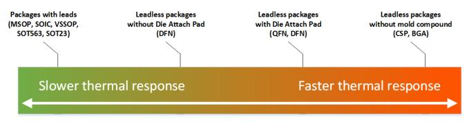
Figure 18. Relative Thermal Response Rate (Typical)
