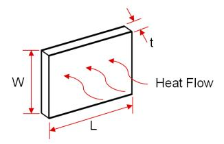
Figure 22. Perpendicular Conduction Heat Flow
