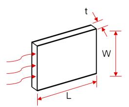
Figure 21. Longitudinal Conduction Heat Flow
