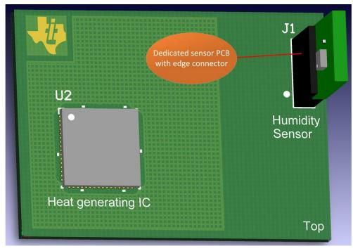
Figure 14. Dedicated Sensor PCB With Edge Connector
