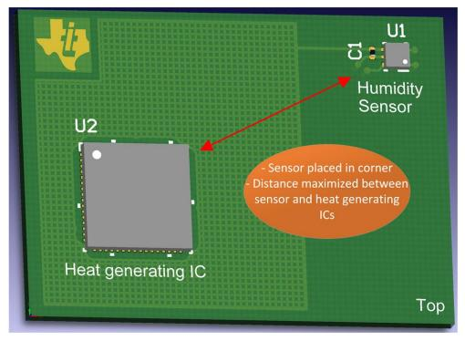
Figure 11. Sensor Placed In PCB Corner
