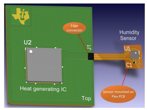
Figure 15. Dedicated Sensor Flex PCB with Edge Connector
