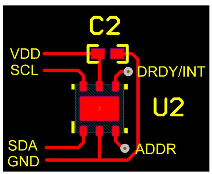
Figure 16. PCB Layout Example HDC1080 [WSON Package]
