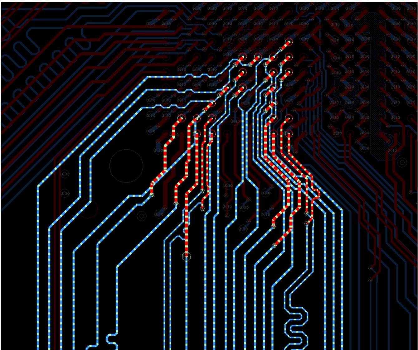
**Figure 4. DDR3 Data Group 1 and 3 Routing**
