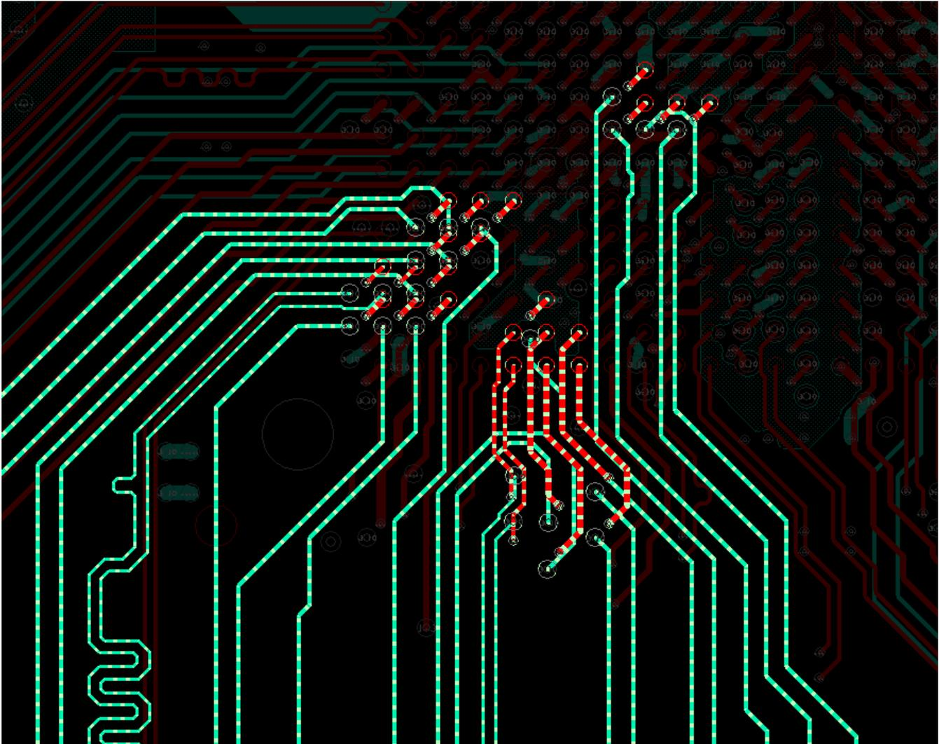
Figure 5. DDR3 Data Group 0 and 2 Routing
