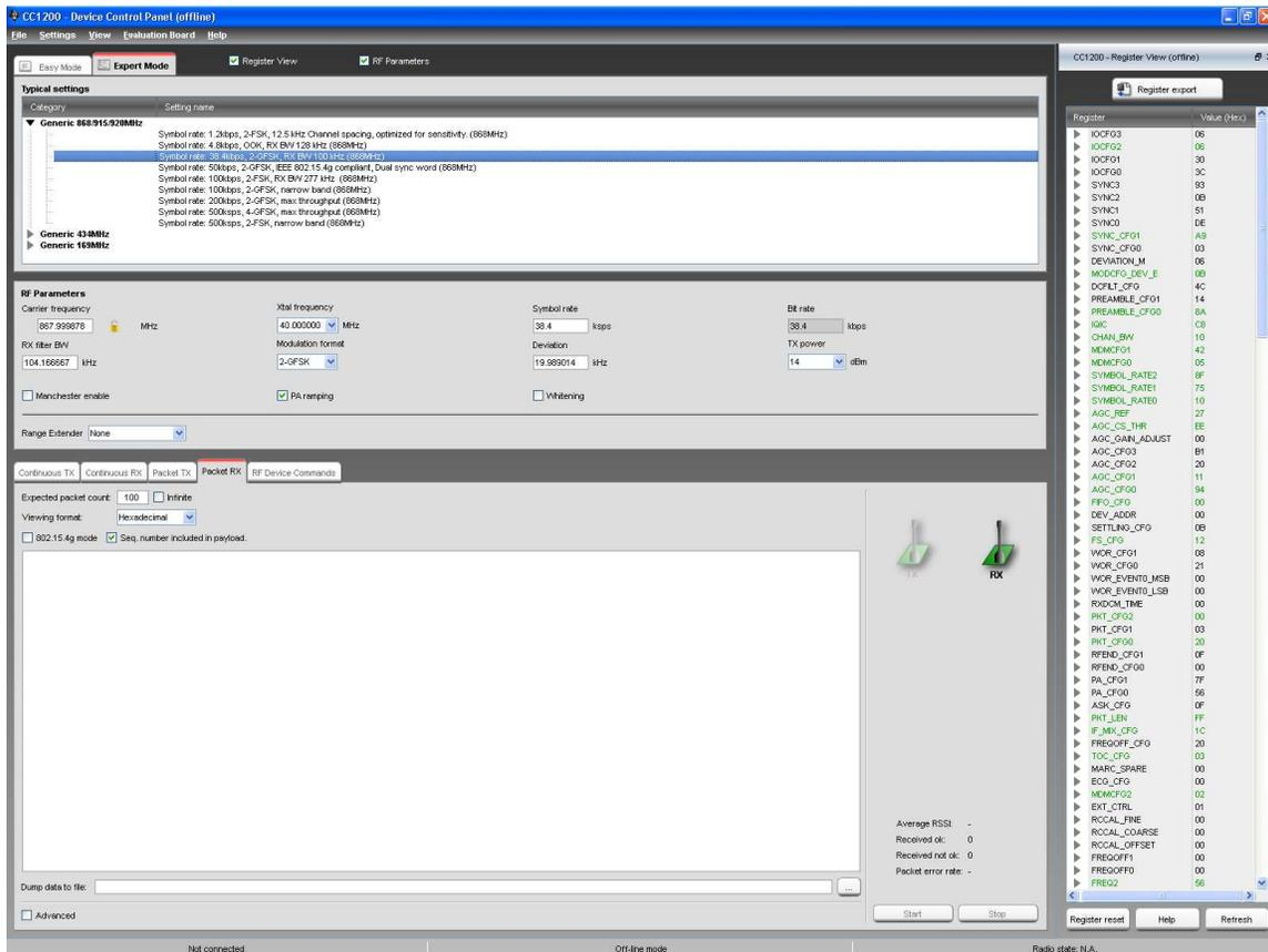
Figure 14. Typical Settings (CC1200, 38.4 kbps, ETSI standard)
