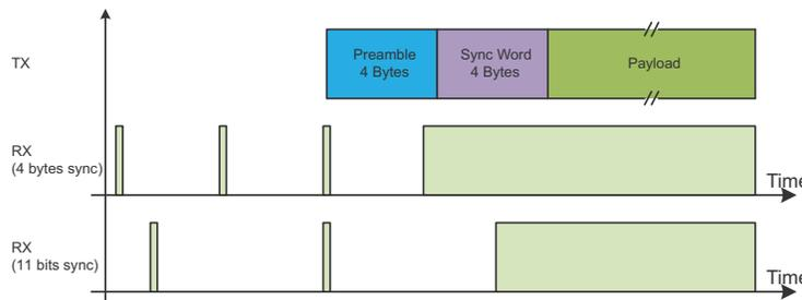
Figure 12. 4 Bytes Sync Word vs. 11 Bits Sync Word
