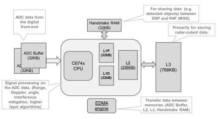
Figure 1. Programmers View of the DSP Subsystem
