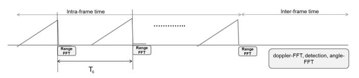
Figure 5. FMCW Frame Structure
