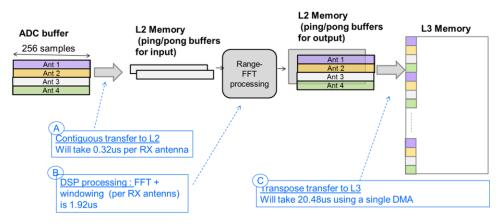
Figure 12. Single-Chirp Use Case Alternate Flow
