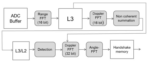
Figure 7. Variant of a Radar Signal Processing Chain
