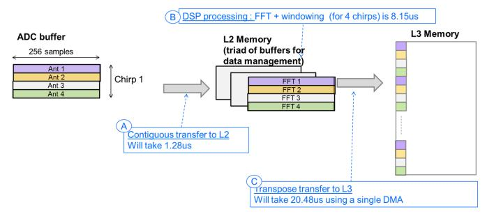
Figure 10. Single-Chirp Use Case
