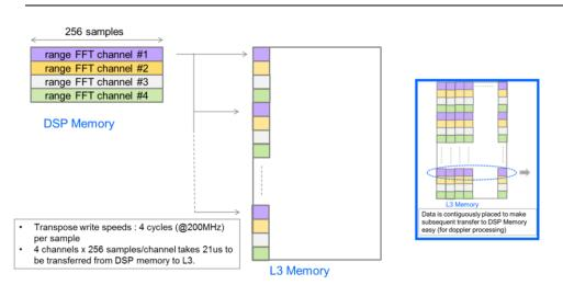
Figure 8. Contiguous-Read Transpose-Write EDMA Access
