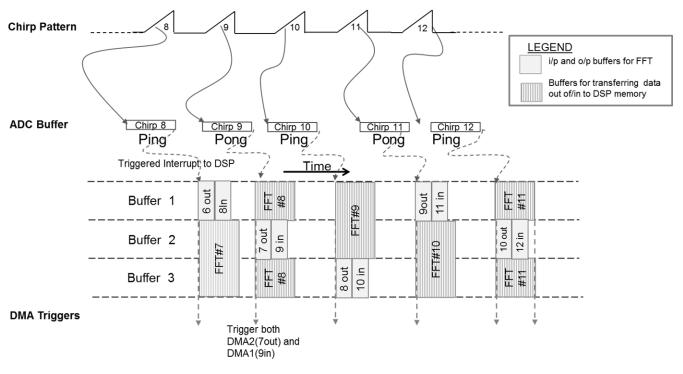
Figure 11. Buffer Management for Data Flow
