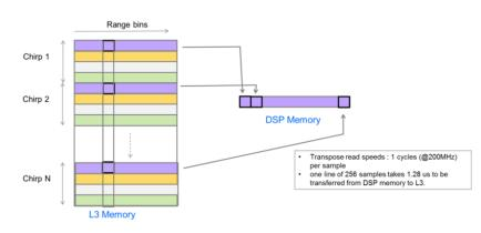
Figure 9. Transpose-Read Contiguous-Write EDMA Access
