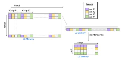
Figure 17. Interframe Processing Case 2
