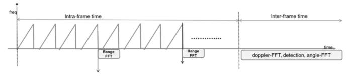
Figure 14. Timing for Multichirp Use Case
