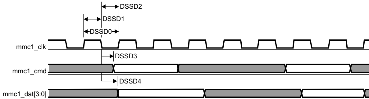
图 7-63. MMC/SD/SDIO in - Default Speed - Transmitter Mode
