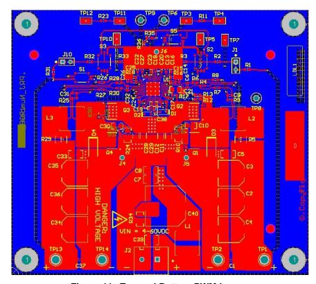
Figure 44. Top and Bottom PWM Layers
