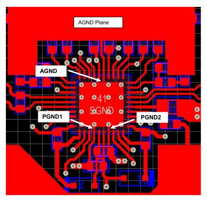
Figure 43. AGND and PGND Connections
