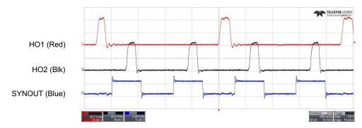
Figure 21. HO1, HO2, and SYNOUT VIN 36 V
