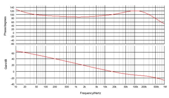
Figure 40. Open Loop Gain and Phase
