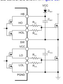
Figure 33. Drivers With Slew Rate Control
