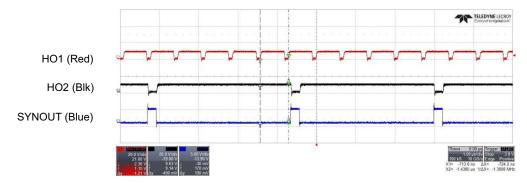
Figure 20. HO1, HO2, SYNOUT VIN 4.2 V
