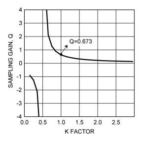
Figure 37. Sampling Gain Q vs K Factor
