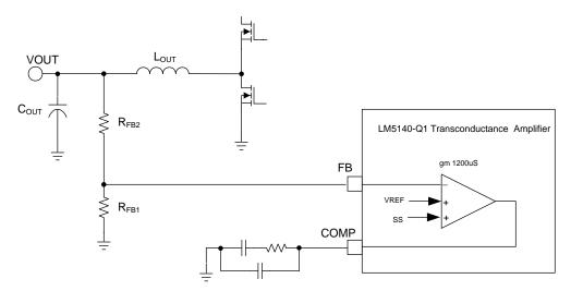
Figure 26. Voltage Feedback
