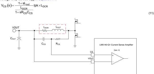
Figure 28. DCR Current Sensing
