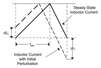
Figure 36. Sub-Harmonic Oscillation
