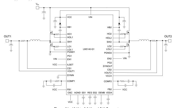
Figure 31. 12-V to 3.3-V and 5-V Converter
