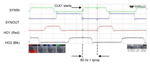
Figure 22. SYNIN and HO1 Timing (2.2 MHz)
