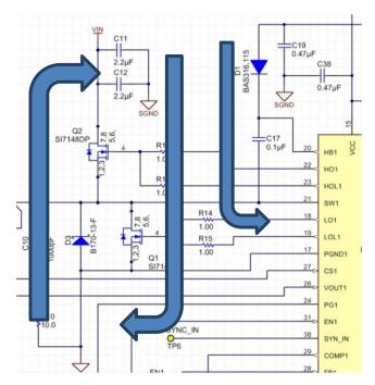
Figure 41. Synchronous Buck Power Flow
