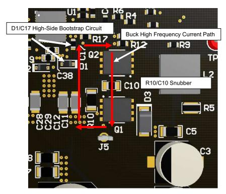
Figure 42. Synchronous Buck High Frequency Current Path
