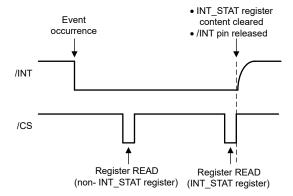
図 8-5. Static INT Assertion Scheme
