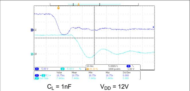
$C_L = 1nF$        $V_{DD} = 12V$
