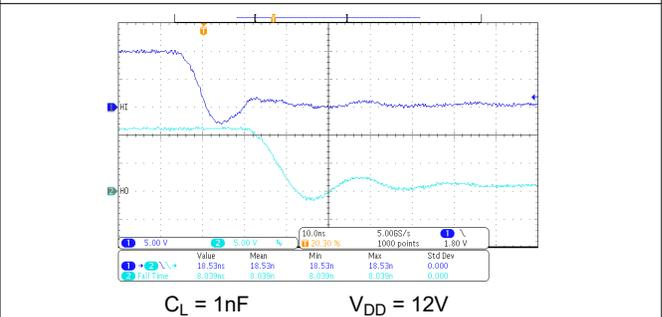
$C_L = 1nF$        $V_{DD} = 12V$
