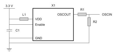
A Legend: L1 = ferrite bead; C1 = 0.1 uF; R1 = 165 ohm / 5%; R2 = 100 ohm / 5%
