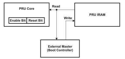
Figure 8. PRU and Boot Controller Block Diagram
