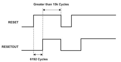
Figure 11. First POR Reset Timing
