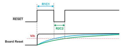
Figure 14. RESET Signal vs Board Reset
