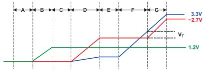
Figure 4. Faulty power-supply ramp
