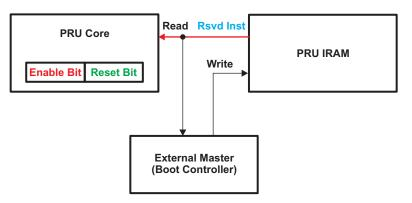
Figure 9. Boot Failure on Power-On
