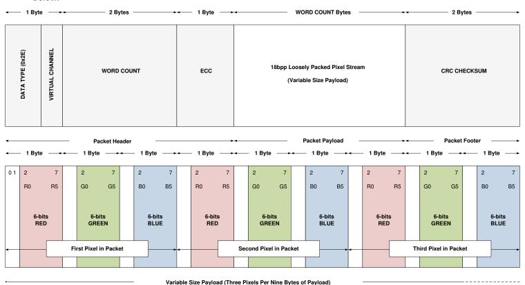
図 8-7. 18 bpp (Loosely Packed) DSI Packet Structure
