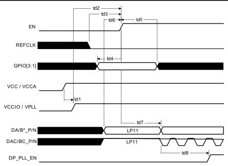
図 7-2. Power-Up Timing Definitions for DPPLL\_CLK\_SRC = DACP/N
