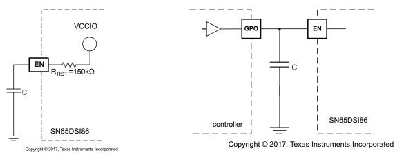
図 8-1. External Capacitor Controlled EN
