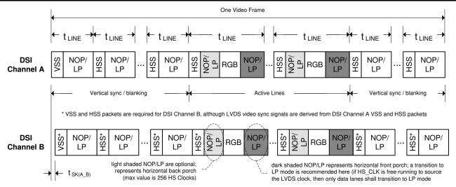
$t_{SK(A\_B)} < 3$  Pixels (72 HS clocks for 18BPP and 24BPP formats)
