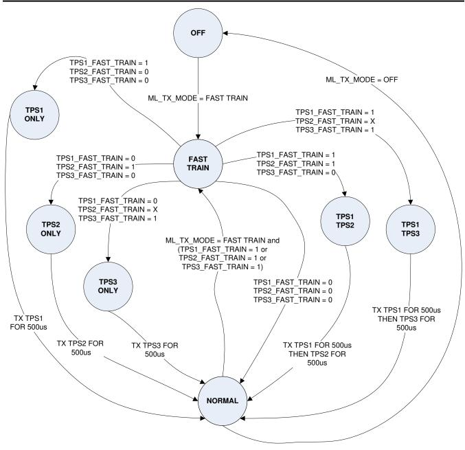
図 8-13. Fast-Link Training State Diagram
