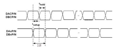
図 7-4. DSI HS Mode Receiver Timing Definitions
