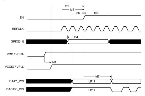
図 7-1. Power-Up Timing Definitions for DPPLL\_CLK\_SRC = REFCLK
