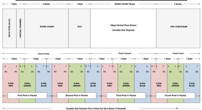
図 8-8. 18 bpp (Tightly Packed) DSI Packet Structure
