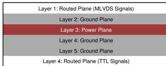
**Figure 25. Six-Layer PCB Board**
