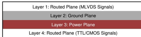
**Figure 24. Four-Layer PCB Board**
