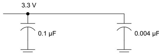
Figure 17. Recommended M-LVDS Bypass Capacitor Layout
