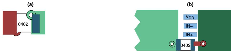
Figure 28. Typical Decoupling Capacitor Layouts
