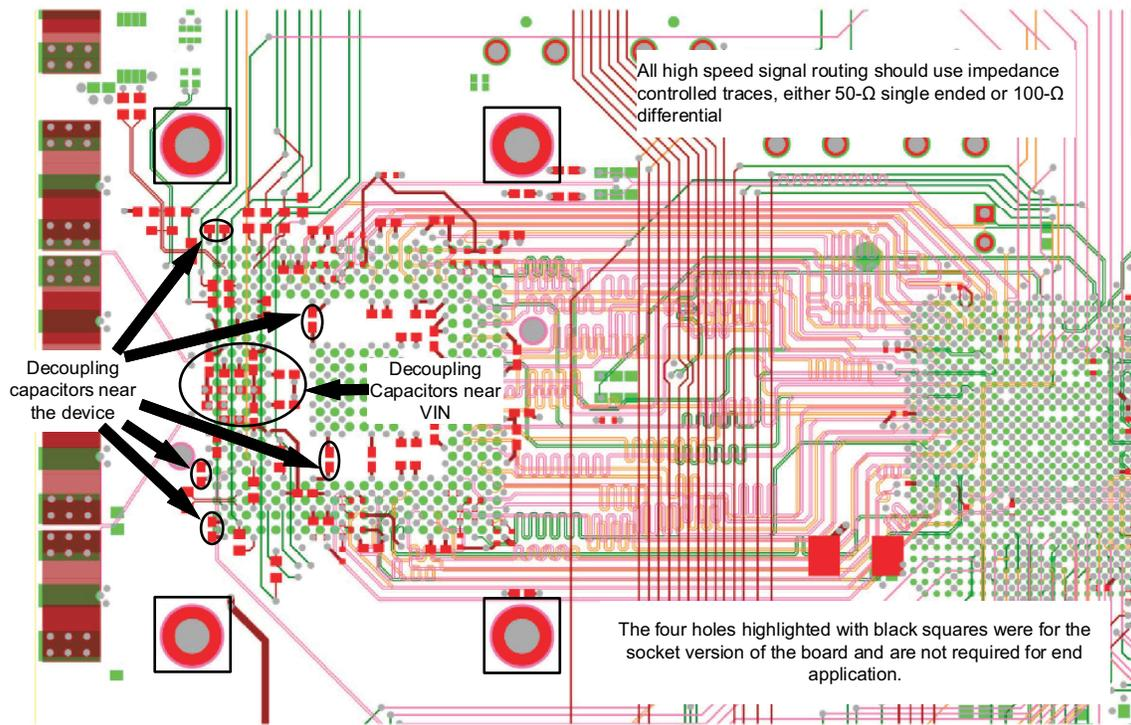
**图 10-3. ADC12D1620 Layout Example: Bottom Side and Inner Layers**
