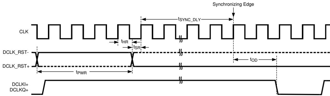
**图 6-7. Data Clock Reset Timing (Demux Mode)**
