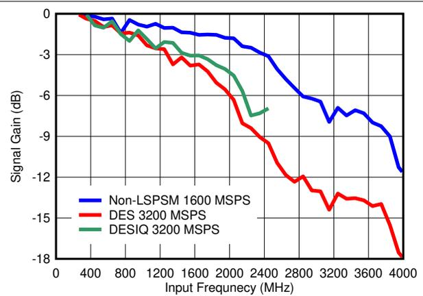
6-38. Insertion Loss vs Input Frequency
