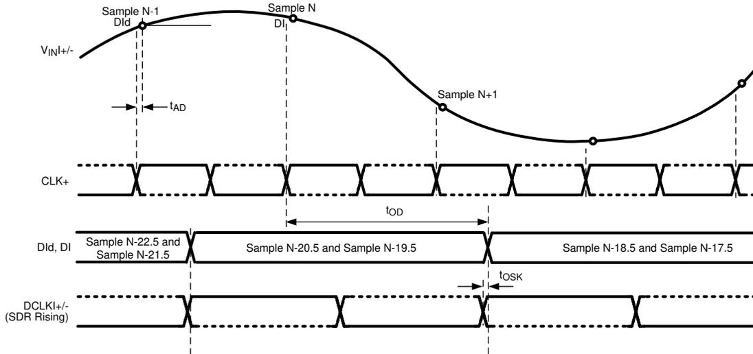
**FIG 6-5. Clocking in LSPSM, 1:2 Demux Mode, Non-DES Mode\***
