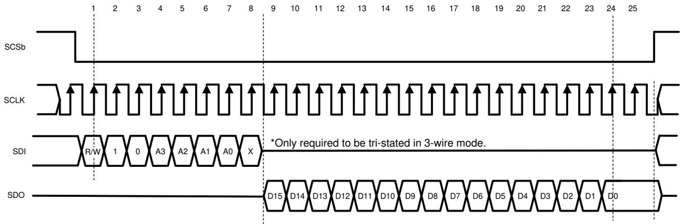
**图 7-3. Serial Data Protocol - Read Operation**
