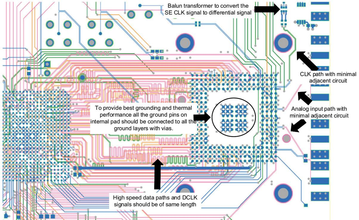
**10-2. ADC12D1620 Layout Example: Top Side and Inner Layers**
