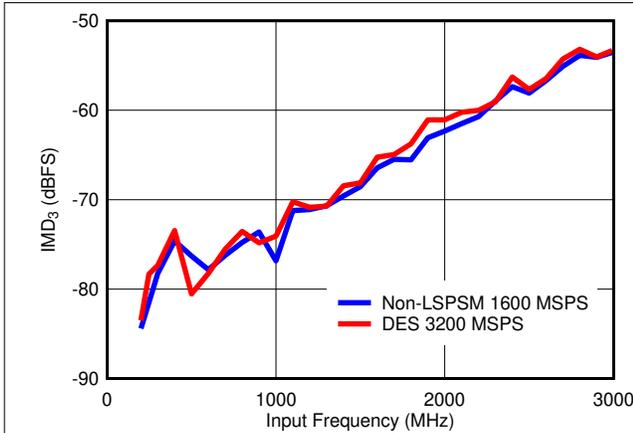
6-35. 3rd Order Intermodulation Distortion vs Input Frequency
