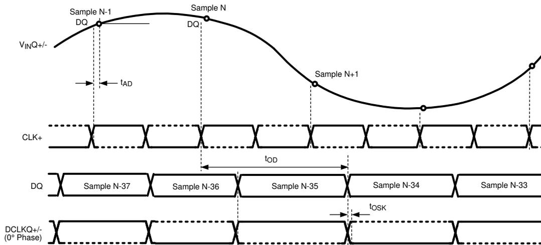
**图 6-2. Clocking in Non-LSPSM, Non-Demux, Non-DES Mode\***
