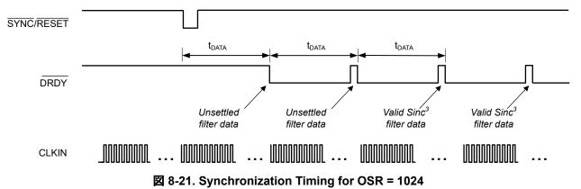
In global-chop mode, conversions are always immediately restarted at the falling edge of the SYNC/RESET pin.
