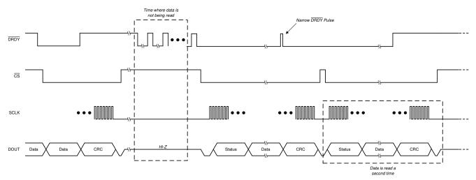
図 8-32. Collecting Data After a Pause by Reading Data Twice
