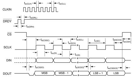
SPI settings are CPOL = 0 and CPHA = 1. CS transitions must take place when SCLK is low.
