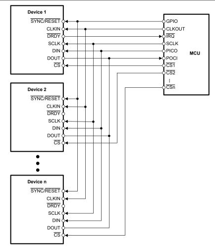
**図** 9-3. Multiple Device Configuration
