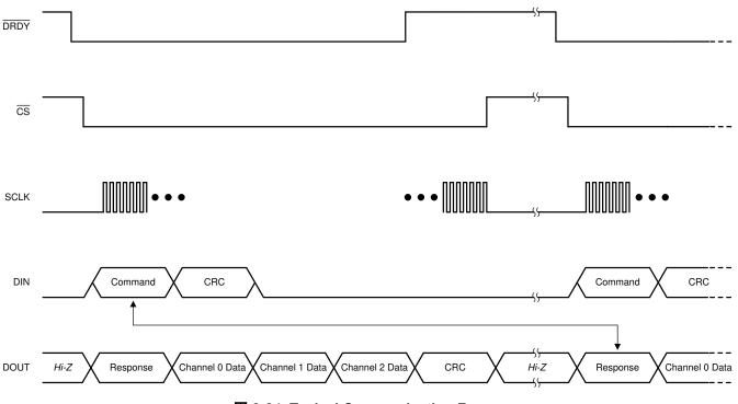
図 8-24. Typical Communication Frame
