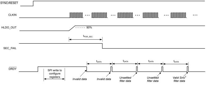
図 8-20. Start-Up Behavior After a Pin Reset and Settling Times
