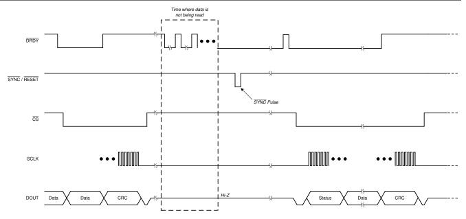
**2**8-31. Collecting Data After a Pause Using the SYNC/RESET Pin
