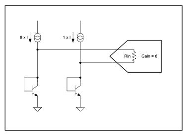
8-15. Internal Temperature Sensor Block Diagram
