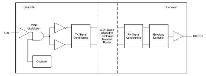
図 8-1. Block Diagram of an Isolation Channel
