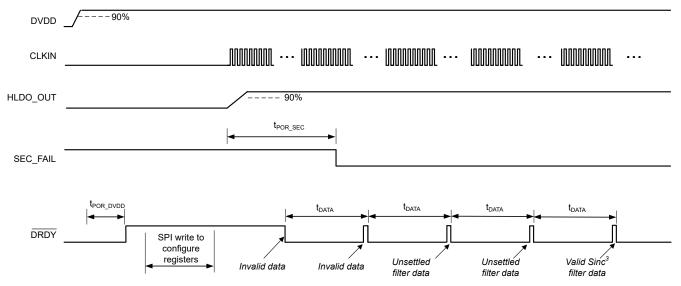
図 8-18. Start-Up Behavior at Power-Up and Settling Times, OSR = 1024
