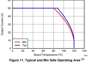
1. The Typical CSD96371Q5M System Characteristic curves are based on measurements made on a PCB design with dimensions of 4.0" (W) x 3.5" (L) x 0.062" (T) and 6 copper layers of 1 oz. copper thickness. See the Application section for detailed explanation.
