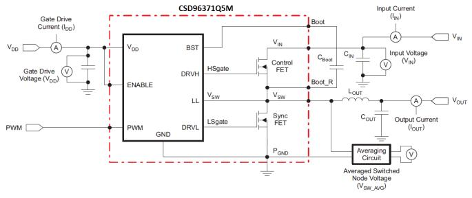
Figure 18. Power Loss Test Circuit
