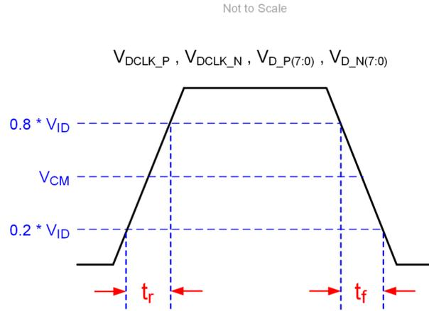
图 6-4. SubLVDS Input Rise and Fall Slew Rate
