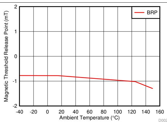
図 2.  $B_{RP}$  Threshold vs Temperature (DRV5015A1-Q1)
