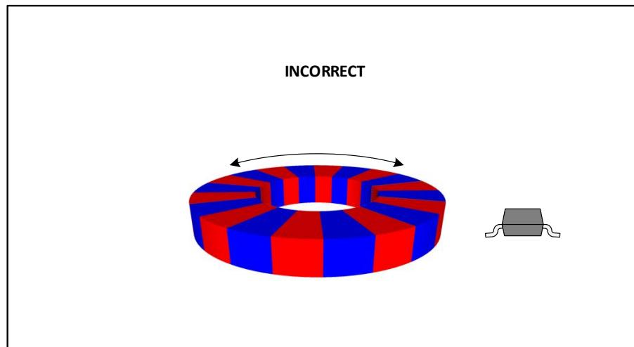
図 22. Correct and Incorrect Magnet Orientations
