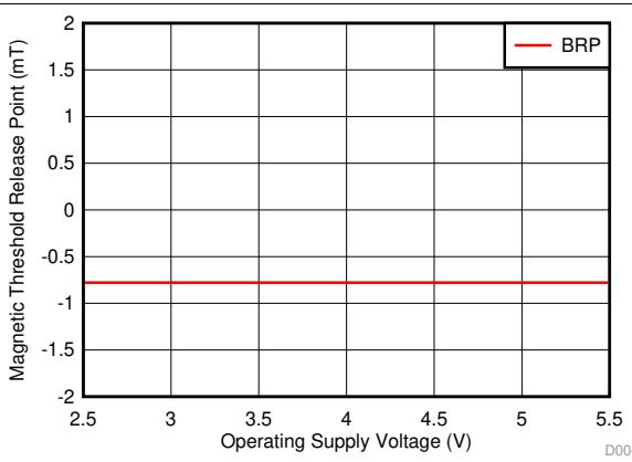
図 4.  $B_{RP}$  Threshold vs Supply Voltage (DRV5015A1-Q1)
