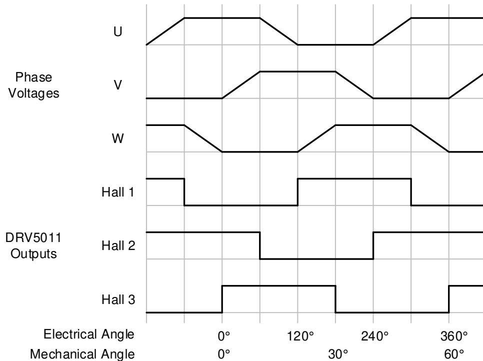
図 19. Phase Voltages and Hall Signals for a 3-Phase BLDC Motor
