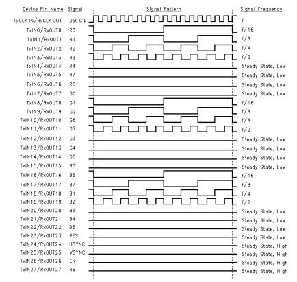
The worst case test pattern produces a maximum toggling of digital circuits, LVDS I/O and CMOS/TTL I/O. The 16 grayscale test pattern tests device power consumption for a "typical" LCD display pattern. The test pattern approximates signal switching needed to produce groups of 16 vertical stripes across the display.
