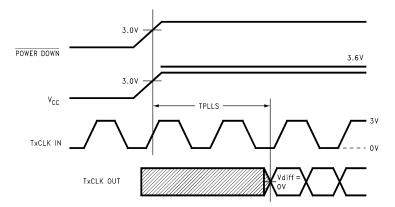
Figure 8. DS90CF383B (Transmitter) Phase Lock Loop Set Time
