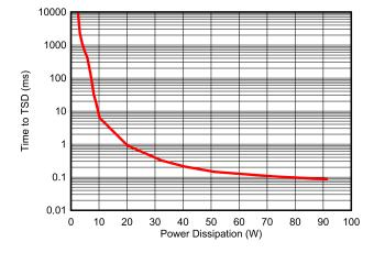
図 8-3. Thermal shut-down plot during inrush
