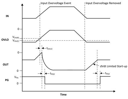
図 7-3. LM73100 Overvoltage Lockout and Recovery
