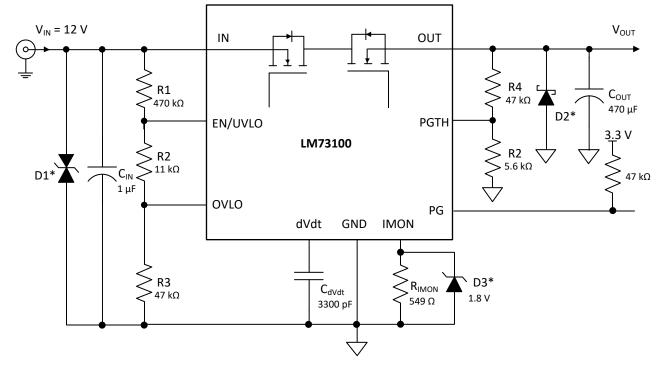
\* Optional circuit components needed for transient protection depending on input and output inductance. Please refer to *Transient Protection* section for details.
