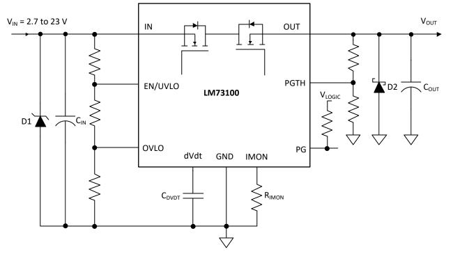
図 9-1. Circuit Implementation with Optional Protection Components
