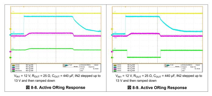
When bus voltages (IN1 and IN2) are matched, device in each rail sees a forward voltage drop and is ON delivering the load current. During this period, current is shared between the rails in the ratio of differential voltage drop across each device.
