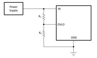
図 7-2. Adjustable Overvoltage Protection
