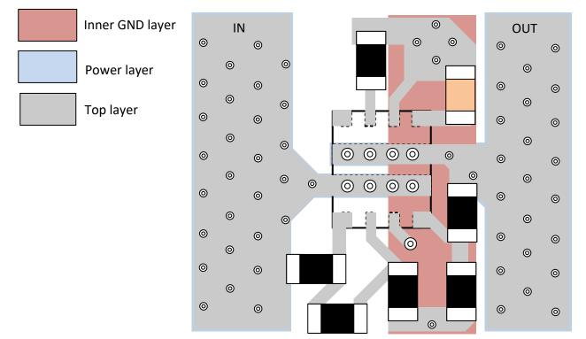
図 10-1. Layout Example - Single LM73100 with PGTH Referred to OUT
