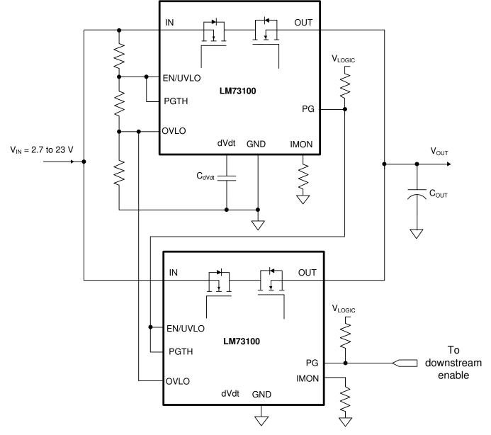
図 8-14. Two Devices Connected in Parallel for Higher Steady State Current Capability
