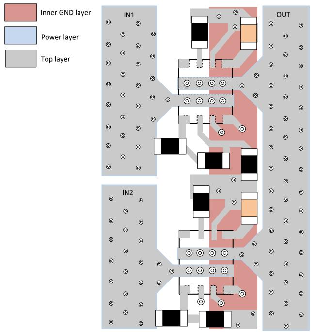
図 10-2. Layout Example - 2 x LM73100 in ORing Configuration
