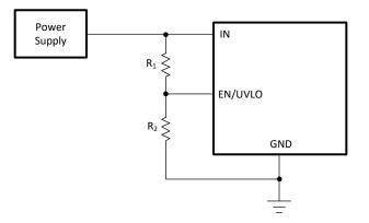
図 7-1. Adjustable Undervoltage Protection
