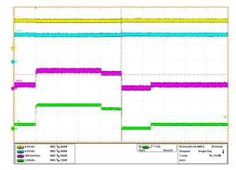
$V_{IN}$  = 12 V,  $C_{OUT}$  = 22  $\mu$ F,  $R_{IMON}$  = 1.15 k $\Omega$ ,  $I_{OUT}$  varied dynamically between 0 A and 3.5 A
