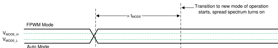
図 7-4. Transition from Auto Mode and FPWM Mode
