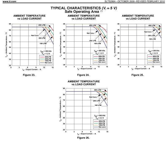
The temperature derating curves represent the conditions at which internal components are at or below the manufacturer's maximum (1) operating temperatures. Derating limits apply to modules soldered directly to a 100 mm x 100 mm double-sided PCB with 2 oz. copper. Please refer to the mechanical specification for more information.
