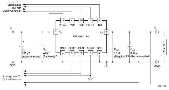
A. [A]  $C_{12}$  and  $C_{O1}$  are optional when the operating frequency is greater than 500 kHz.
