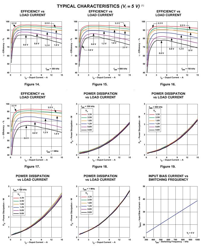
(1) The electrical characteristic data has been developed from actual products tested at 25°C. This data is considered typical for the converter.
