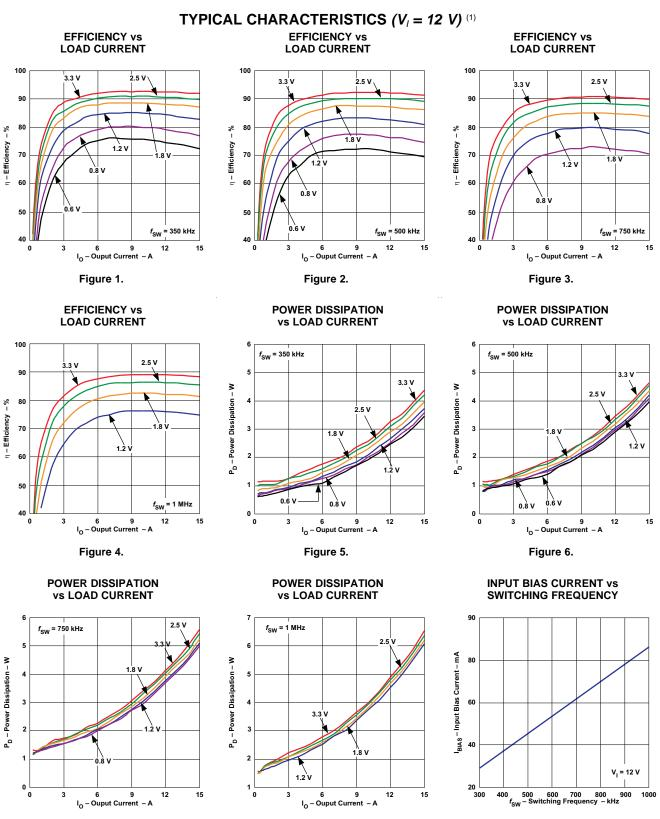
The electrical characteristic data has been developed from actual products tested at 25°C. This data is considered typical for the converter.
