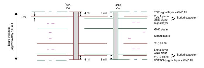
図 27. Low Inductance, High-Capacitance Power Connection
