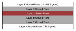
図 25. Six-Layer PCB Board
