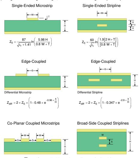
図 19. Controlled-Impedance Transmission Lines
