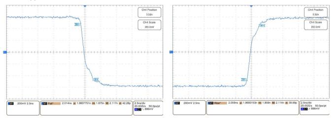
$V_{CC} = 3.3 \text{ V}$   $T_A = 25^{\circ}\text{C}$  20. Driver Fall Time
