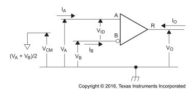
図 10. Receiver Voltage and Current Definitions
