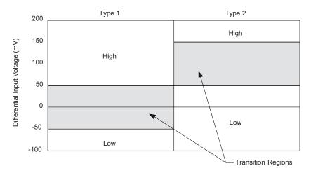
図 18. Expanded Graph of Receiver Differential Input Voltage Showing Transition Region
