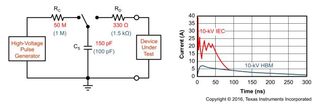
図 15. HBM and IEC-ESD Models and Currents in Comparison (HBM Values in Parenthesis)
