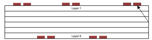
図 29. Staggered Trace Layout
