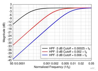
図 8-17. HPF Filter Frequency Response Plot
