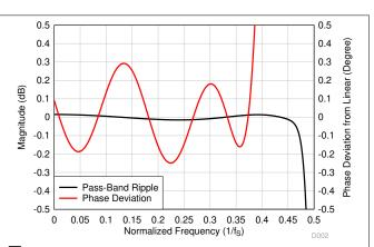
図 8-44. Low-Latency Decimation Filter Pass-Band Ripple and Phase Deviation
