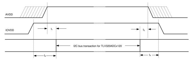
**図 10-1. Power-Supply Sequencing Requirement Timing Diagram**
