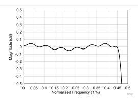
図 8-28. Linear Phase Decimation Filter Pass-Band Ripple
