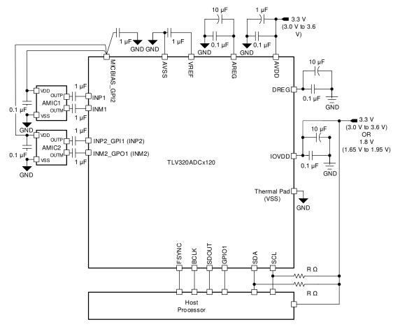
図 9-1. Two-Channel Analog Microphone Recording Diagram
