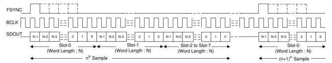
図 8-1. TDM Mode Standard Protocol Timing (TX OFFSET = 0)
