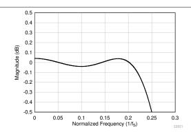
図 8-34. Linear Phase Decimation Filter Pass-Band Ripple
