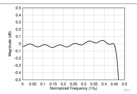
図 8-26. Linear Phase Decimation Filter Pass-Band Ripple
