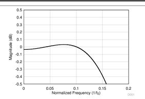
図 8-36. Linear Phase Decimation Filter Pass-Band Ripple
