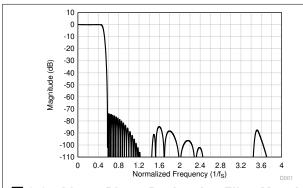
図 8-27. Linear Phase Decimation Filter Magnitude Response
