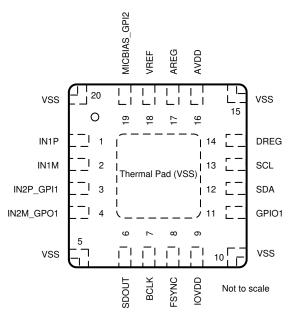
図 6-1. RTE Package, 20-Pin WQFN With Exposed Thermal Pad, Top View
