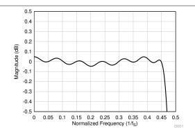
図 8-24. Linear Phase Decimation Filter Pass-Band Ripple
