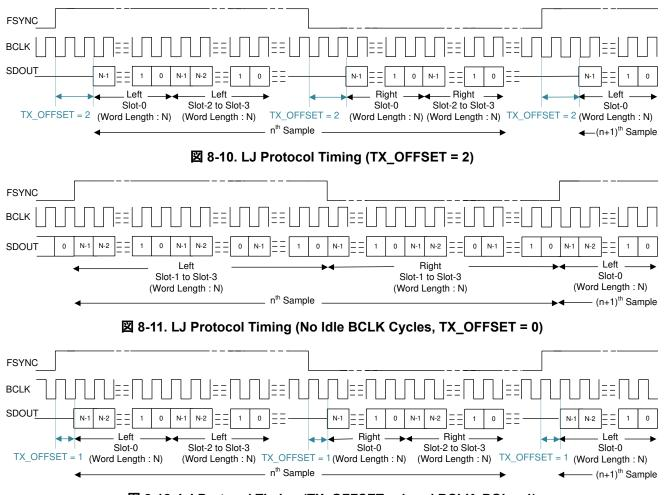
図 8-12. LJ Protocol Timing (TX\_OFFSET = 1 and BCLK\_POL = 1)
