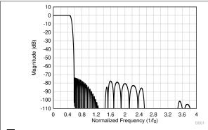
図 8-25. Linear Phase Decimation Filter Magnitude Response
