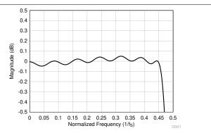
図 8-22. Linear Phase Decimation Filter Pass-Band Ripple
