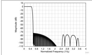
図 8-21. Linear Phase Decimation Filter Magnitude Response
