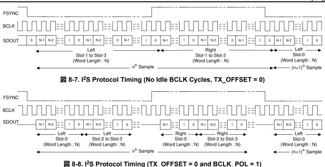
For proper operation of the audio bus in I<sup>2</sup>S mode, the number of bit clocks per frame must be greater than or equal to the number of active output channels (including left and right slots) times the programmed word length
