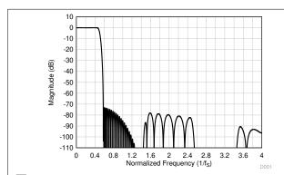
図 8-23. Linear Phase Decimation Filter Magnitude Response
