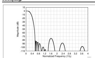
図 8-35. Linear Phase Decimation Filter Magnitude Response
