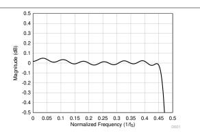
図 8-20. Linear Phase Decimation Filter Pass-Band Ripple
