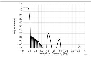
図 8-31. Linear Phase Decimation Filter Magnitude Response
