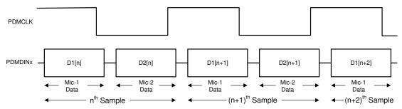
図 8-65. Digital PDM Microphone Protocol Timing Diagram
