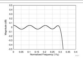
図 8-32. Linear Phase Decimation Filter Pass-Band Ripple
