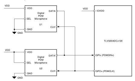
図 8-64. Digital PDM Microphones Connection Diagram for the TLV320ADC5120
