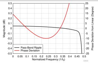
図 8-50. Ultra-Low-Latency Decimation Filter Pass-Band Ripple and Phase Deviation
