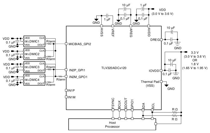
図 9-6. Four-Channel Digital PDM Microphone Recording Diagram
