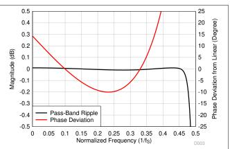
図 8-52. Ultra-Low-Latency Decimation Filter Pass-Band Ripple and Phase Deviation
