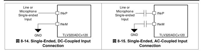
The device allows for flexibility in choosing the typical input impedance on INxP or INxM from 2.5 kΩ (default), 10 kΩ, and 20 kΩ based on the input source impedance. The higher input impedance results in slightly higher noise or lower dynamic range.  $\frac{1}{8}$  8-9 lists the configuration register settings for the input impedance for the record channel.
