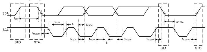
☑ 7-1. I<sup>2</sup>C Interface Timing Diagram
