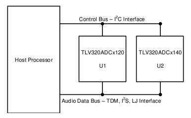
図 8-13. Multiple Devices With Shared Control and Audio Data Buses
