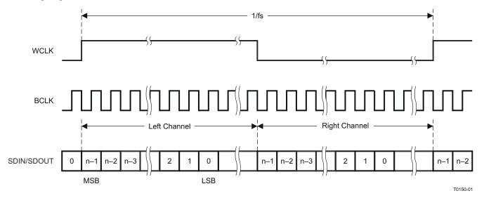
図 10-4. Left-Justified Serial Data Bus Mode Operation
