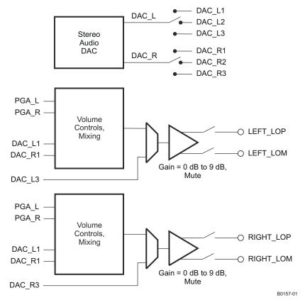
2 10-15. Architecture of the Output Stage Leading to the Fully Differential Line Output Drivers
