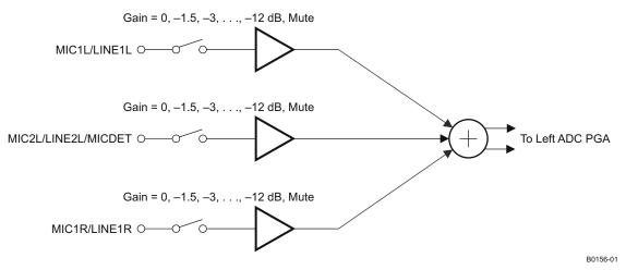
図 10-14. Left-Channel, Single-Ended Analog Input Mixing Configuration
