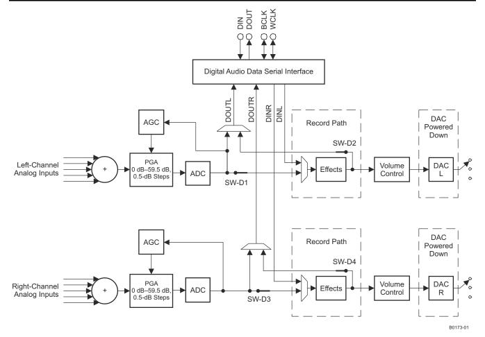
**2** 10-22. Record-*Only* Mode With Digital Processing Path Enabled
