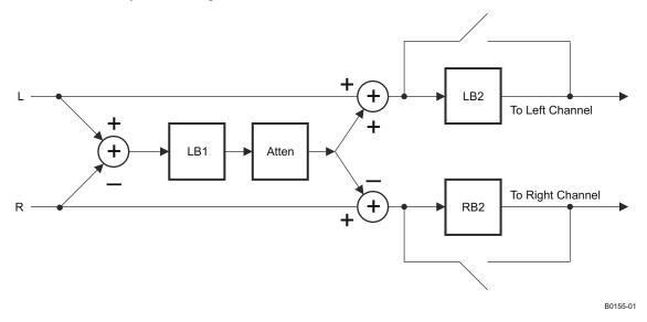
2 10-11. Architecture of the Digital Audio Processing When 3-D Effects Are Enabled
