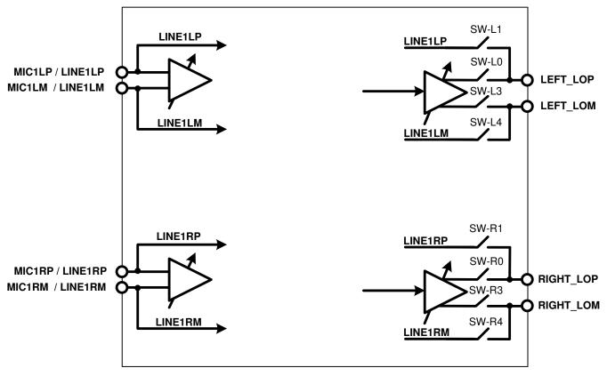
図 10-21. Passive Analog Bypass Mode Configuration
