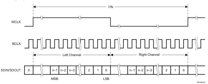
図 10-3. Right-Justified Serial Data Bus Mode Operation
