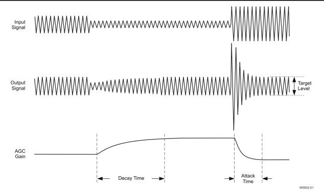
図 10-9. Typical Operation of the AGC Algorithm During Speech Recording
