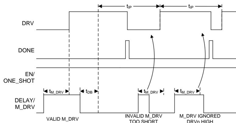
**Figure 11. Manual Power ON in Timer Mode**
