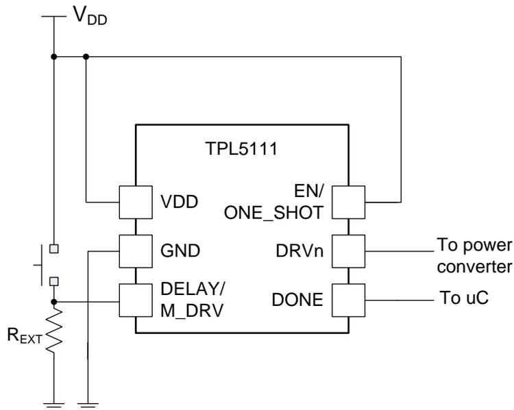
**Figure 13. Manual Power ON With SPST Switch**
