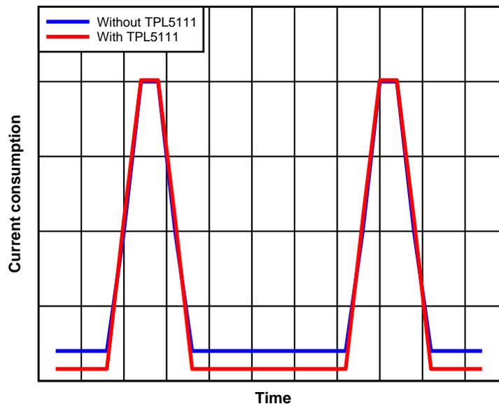
Figure 15. Effect of TPL5111 on Current Consumption
