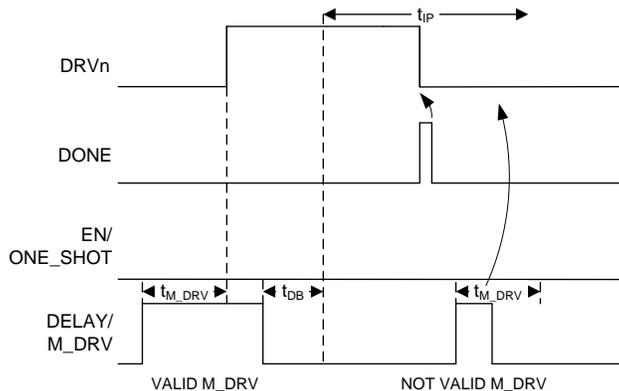
Figure 12. Manual Power ON in One-Shot Mode
