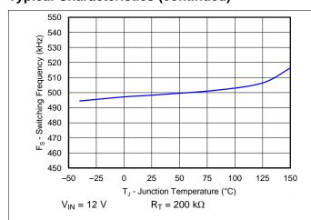
Figure 5. Switching Frequency vs Junction Temperature
