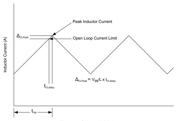
Figure 24. Current Limit Delay
