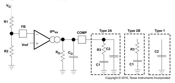
Figure 31. Types of Frequency Compensation
