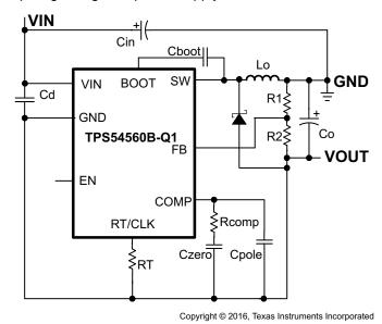
Figure 56. TPS54560B-Q1 Inverting Power Supply from SLVA317 Application Note
