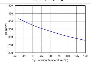
Figure 8. EA Transconductance vs Junction Temperature
