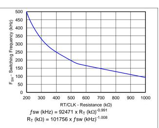
Figure 6. Switching Frequency vs RT/CLK Resistance Low Frequency Range
