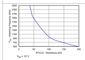
Figure 7. Switching Frequency vs RT/CLK Resistance
