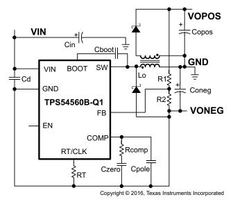
Figure 57. TPS54560B-Q1 Split Rail Power Supply
