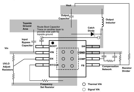
Figure 58. PCB Layout Example
