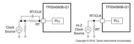
Figure 25. Synchronizing to a System Clock
