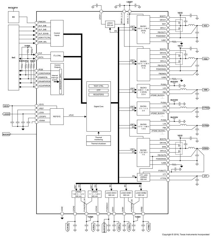
Figure 1-1. PMIC Functional Block Diagram
