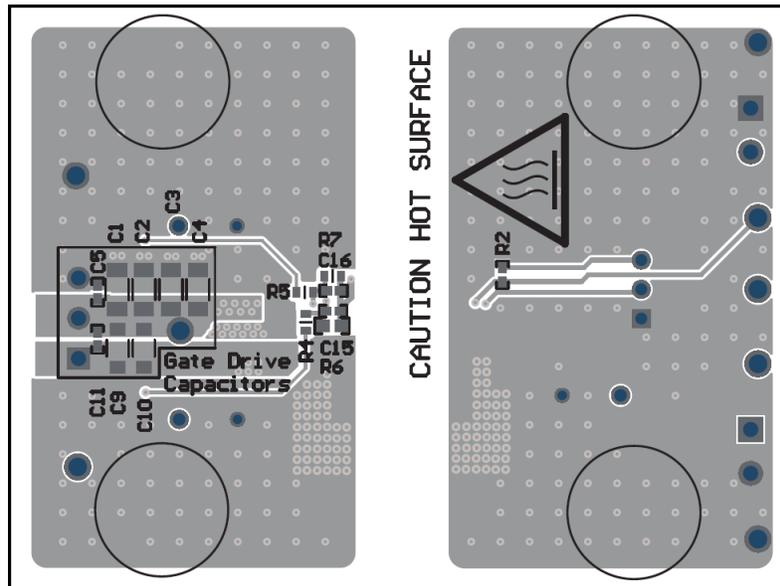
図 8-24. UCC14341-Q1EVM, PCB Bottom Layer, Assembly (Mirrored View)
