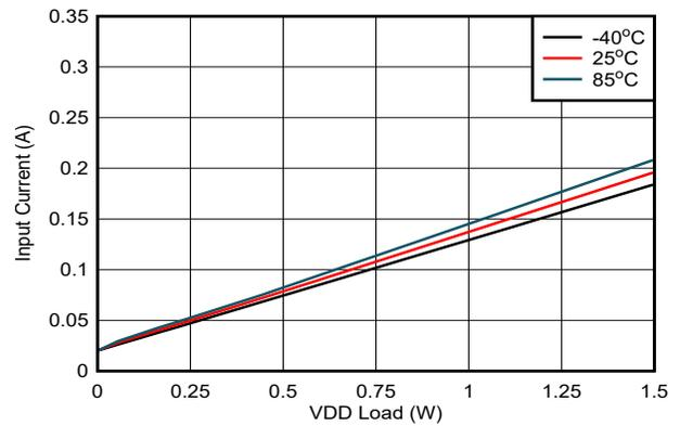
图 6-23. Input Current vs. Load on  $V_{DD-VEE}$ :  $V_{IN} = 15V$ ,  $V_{DD-VEE} = 22V$ ,  $V_{COM-VEE} = 4V$ , No Load on  $V_{COM-VEE}$
