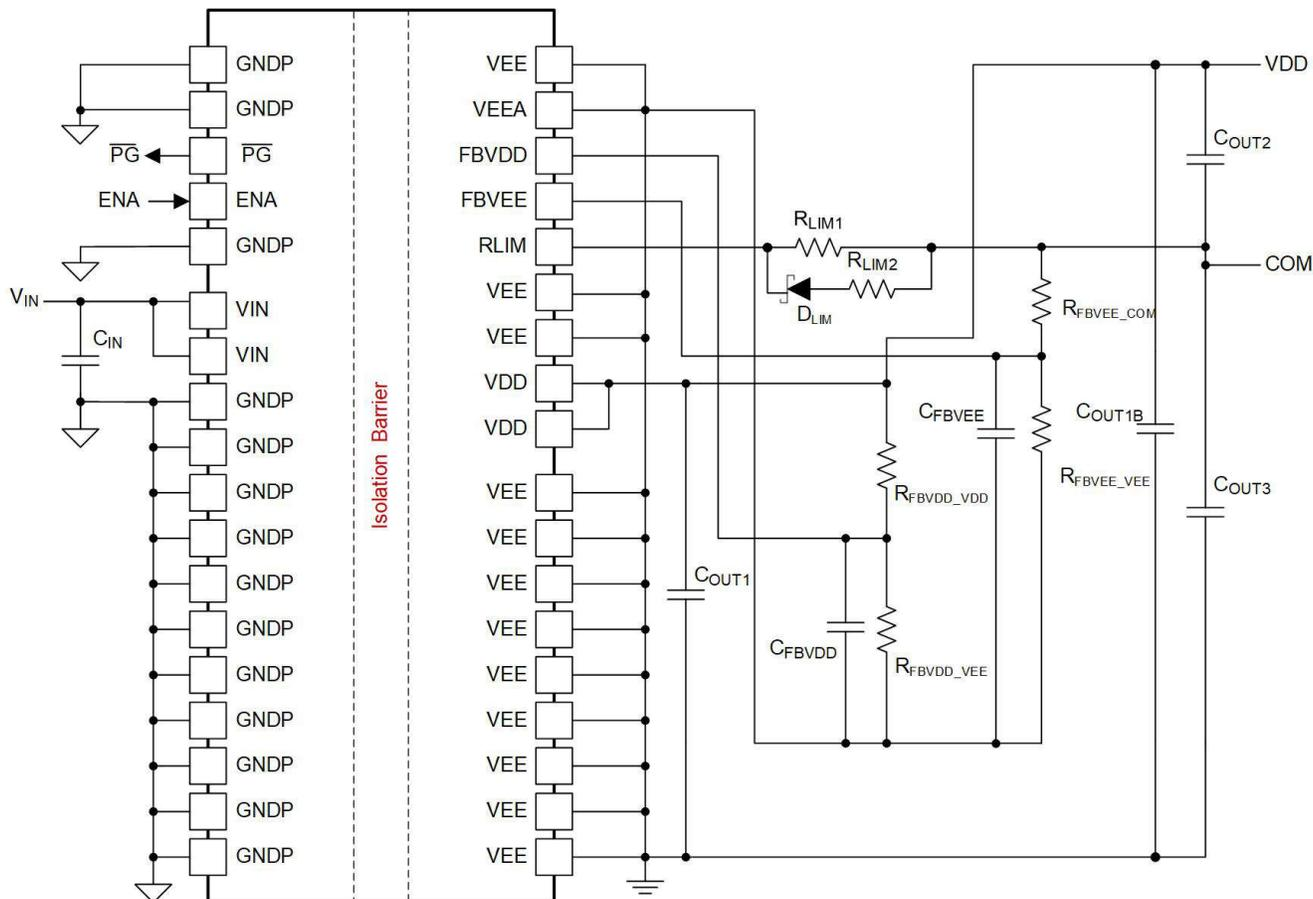
8-8. Dual output application schematic configured for  $V_{COM\_VEE}$  regulation > 2.5V
