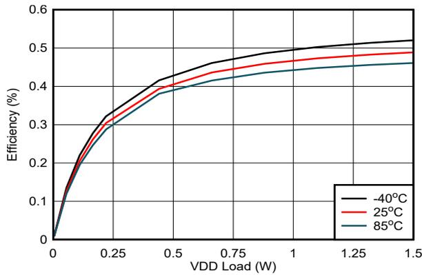
图 6-20. Efficiency vs. Load on  $V_{DD-VEE}$ :  $V_{IN} = 16.5V$ ,  $V_{DD-VEE} = 22V$ ,  $V_{COM-VEE} = 4V$ , No Load on  $V_{COM-VEE}$
