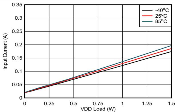
图 6-24. Input Current vs. Load on  $V_{DD-VEE}$ :  $V_{IN} = 16.5V$ ,  $V_{DD-VEE} = 22V$ ,  $V_{COM-VEE} = 4V$ , No Load on  $V_{COM-VEE}$
