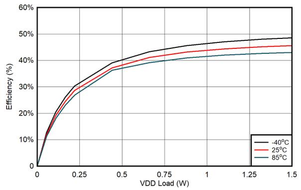
图 6-21. Efficiency vs. Load on  $V_{DD-VEE}$ :  $V_{IN} = 18V$ ,  $V_{DD-VEE} = 22V$ ,  $V_{COM-VEE} = 4V$ , No Load on  $V_{COM-VEE}$
