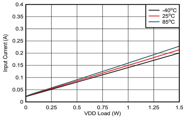
图 6-22. Input Current vs. Load on  $V_{DD-VEE}$ :  $V_{IN} = 13.5V$ ,  $V_{DD-VEE} = 22V$ ,  $V_{COM-VEE} = 4V$ , No Load on  $V_{COM-VEE}$
