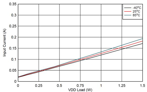
图 6-25. Input Current vs. Load on  $V_{DD-VEE}$ :  $V_{IN} = 18V$ ,  $V_{DD-VEE} = 22V$ ,  $V_{COM-VEE} = 4V$ , No Load on  $V_{COM-VEE}$
