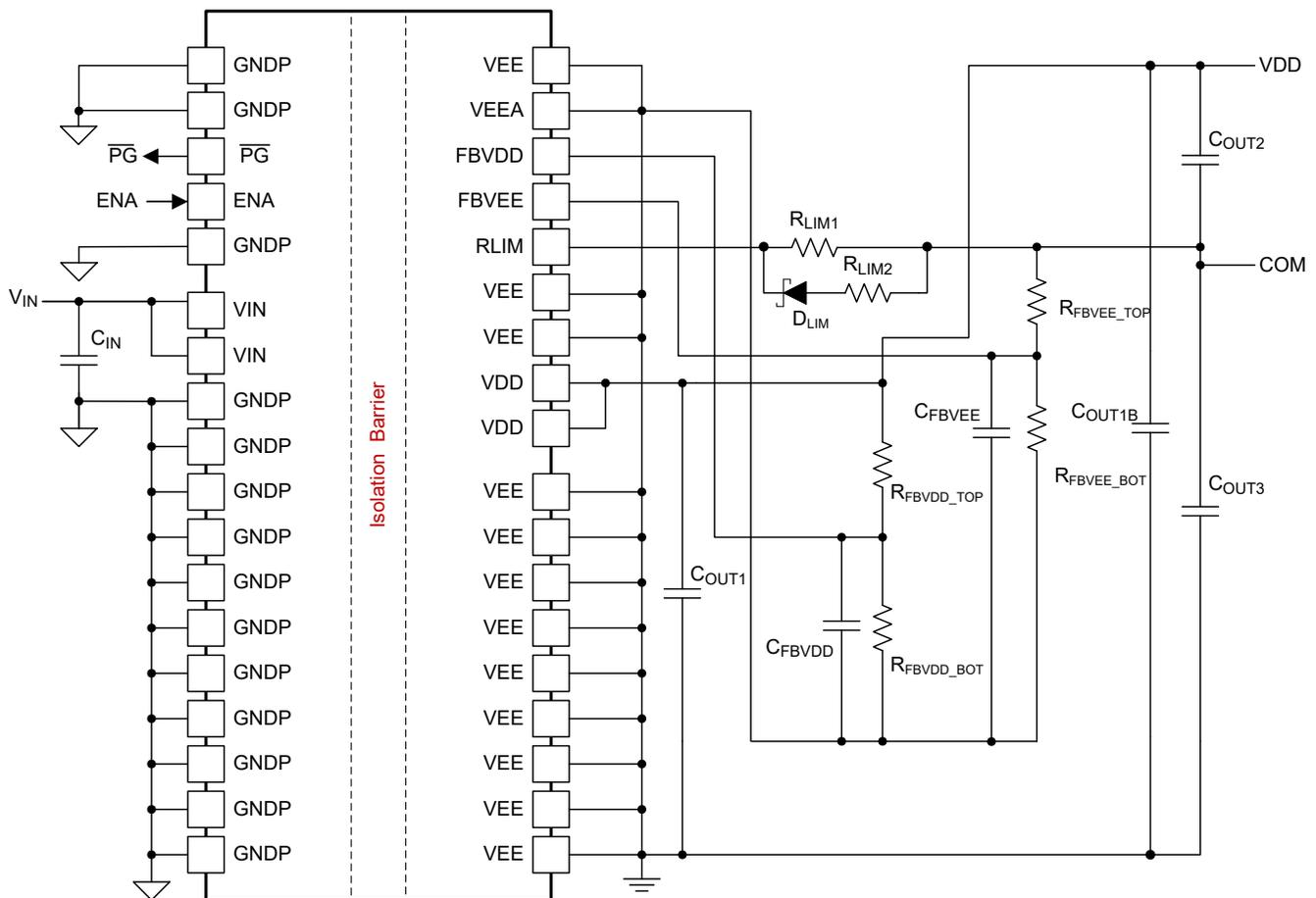
図 8-1. Dual Adjustable Output Configuration
