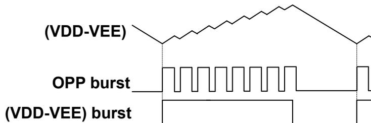
図 7-4. Diagram of Over-Power-Protection with Baby Burst
