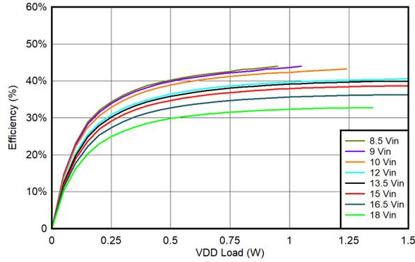
図 6-32. UCC14341B-Q1 Efficiency vs. Load on  $V_{DD-VEE}$ :  $T_{AMBIENT} = 85^{\circ}C$ ,  $V_{VDD-VEE} = 15V$ ,  $V_{COM-VEE} = 4V$ , No Load on  $V_{COM-VEE}$
