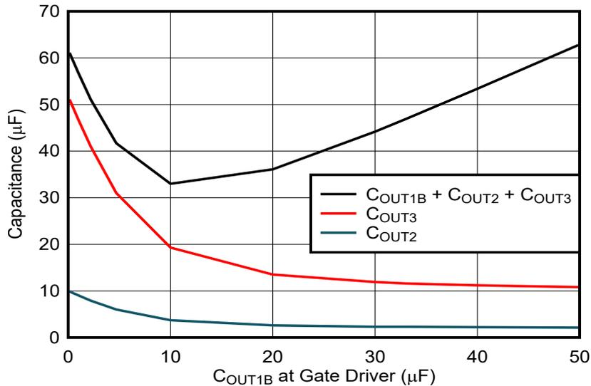
图 8-5. Output Capacitance Variation with  $C_{out1B}$  selection
