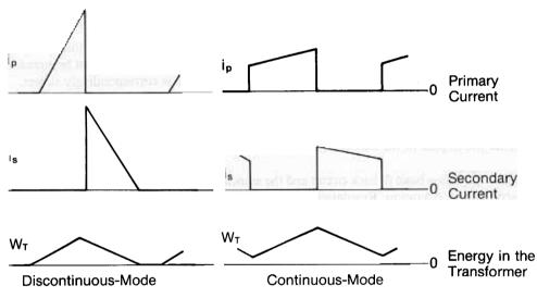
Figure 2. Discontinuous vs Continuous Flyback Waveforms
