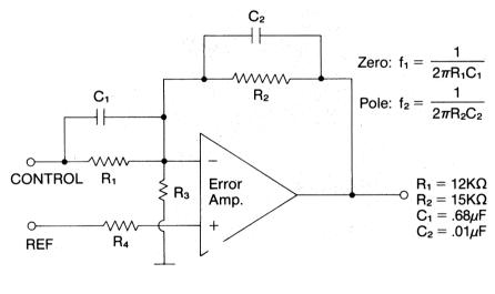
Figure 8. Error Amplifier with Compensation
