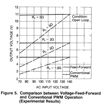
The UC3840 IC provides a terminal which can be used to clamp the control signal internally to any desired level. When used in conjunction with the feed-forward circuitry, this feature allows the designer to set an upper limit on the transformer "volt-second" product. The design of the transformer can then be further optimized for size and cost.
