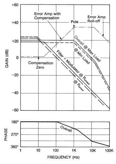
The resulting frequency response is illustrated in Figure 7A.
