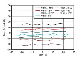
Figure 4. Total Error (LSB) for Different V<sub>cm</sub> and V<sub>diff</sub> When Using Solution 2
