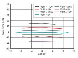
Figure 6. Total Error (LSB) for Different V $_{\rm cm}$  and V $_{\rm diff}$  When Using Solution 3
