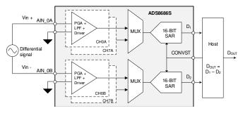
Figure 5. Capturing Differential Signal Inputs as two Single-Ended Signals Using the Dual Simultaneous Sampling SAR ADCs of the ADS8686S
