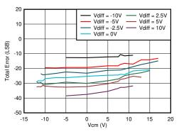
Figure 2. Total Error (LSB) for Different V<sub>cm</sub> and V<sub>diff</sub> When Using Solution 1
