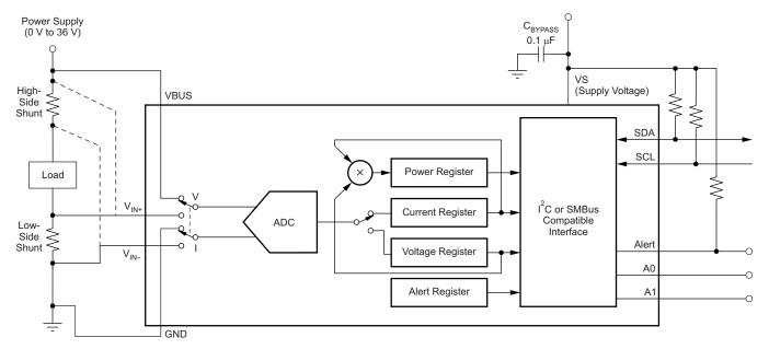
Figure 1. Functional Block Diagram
