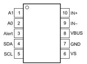
Figure 2. Pin Diagram
