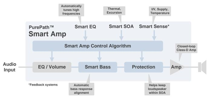
Figure 1. PurePath<sup>™</sup> Smart Amp Block Diagram
