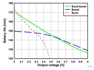
Figure 3. Battery Lifetime vs. Output Voltage: Constant Current Load (1 A)
