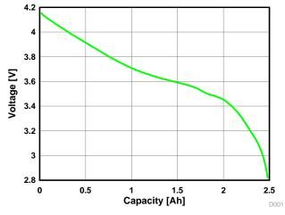
Figure 1. Discharge Profile of a Li-ion Battery at 1 A
