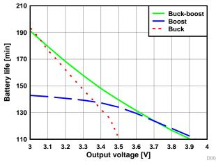
Figure 4. Battery Lifetime vs. Output Voltage: Resistive Load (3.6  $\Omega$ )
