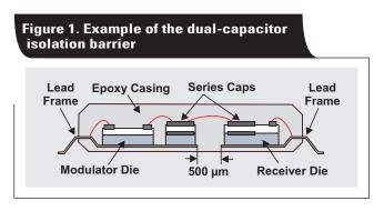
and CSA standards. As shown in Figure 1, the isolation barrier of this device is constructed with two series capacitors, each having an equivalent of basic insulation through a silicon dioxide (SiO<sub>2</sub>) layer of 13.5  $\mu$ m (27  $\mu$ m total). The surge immunity is rated to ±10,000 V and the working voltage is 1500 VDC and 1000 V<sub>RMS</sub>, respectively.
