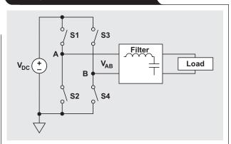
can range from 10 to 200 kHz, depending on the application and type of switch. In Figure 3a, the duty cycle at node A is more than 50% and in Figure 3b, the duty cycle is less than 50% at node B. This creates a positive voltage across the load as shown in Figure 3c.
