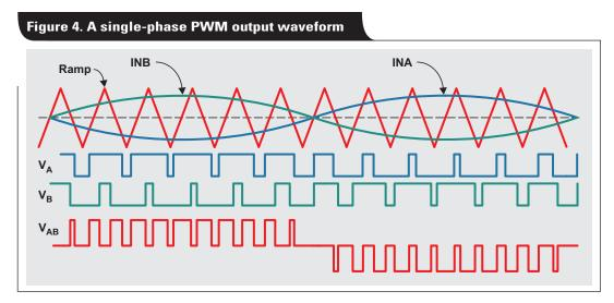
Controlling the duty cycle,  $D_A$  and  $D_B$ , allows control of the output voltage,  $V_{AB}$ . A sinusoidal single-phase PWM waveform is obtained by comparing a reference sine wave INA and INB with a high-frequency triangular signal as shown in Figure 4.
