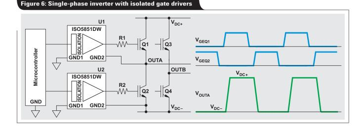
ISO5851 datasheet, Figure 7 shows a typical application diagram. The Ready (RDY) and Fault (FLT) pins are pulled up by 10-k $\Omega$  resistors. These resistor values may need to be lower for noise immunity. Transient noise can generate a false fault or low under-voltage lockout (UVLO) signal. This issue can be solved by either reducing the resistor values or increasing the capacitance of C1 and C2.
