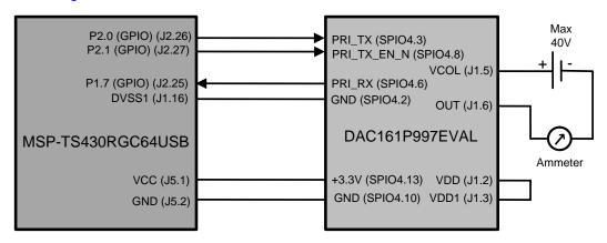
Figure 2. DAC161P997 to MSP430 Connection Diagram
