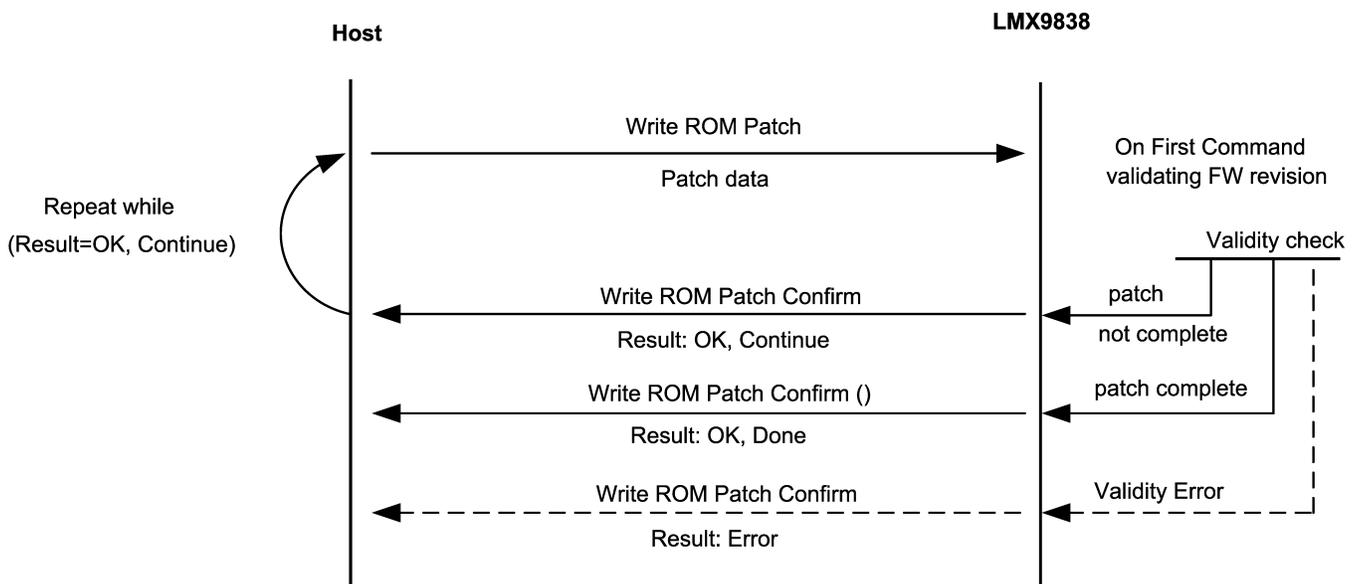
**Figure 2. Write ROM Patch Flow**
