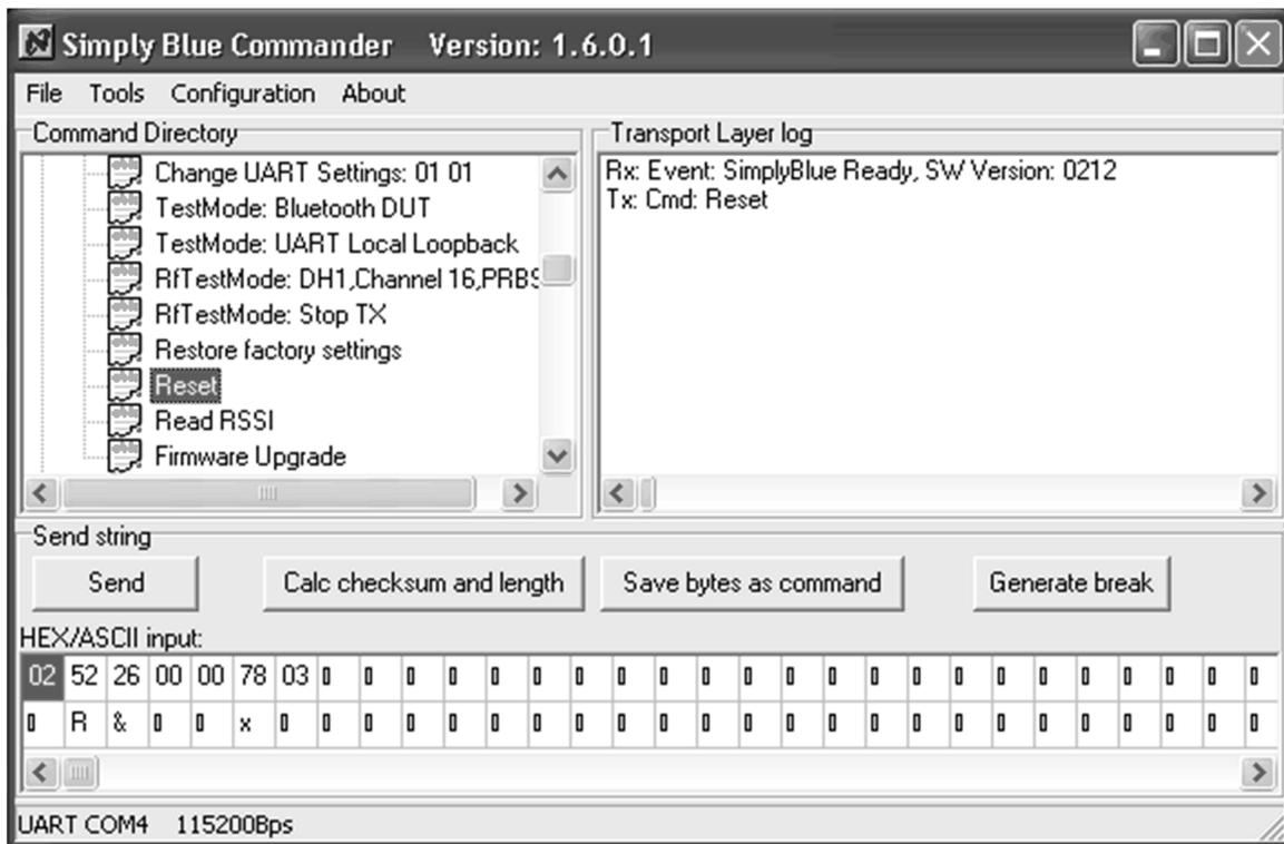
Figure 1. “SimplyBlue Ready” in Simply Blue Commander
