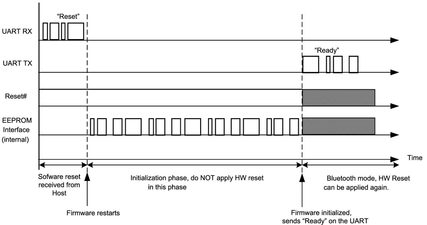
**Figure 4. Safe Reset Timing on Software Reset**
