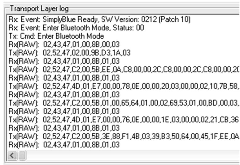
**Figure 6. Step 2/3, Apply Patch 10 and Enter BT\_Mode**
