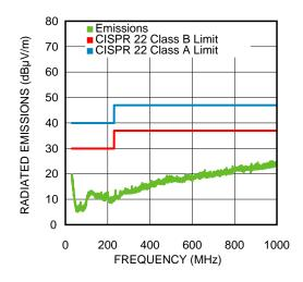
Figure 3. CISPR 22 Radiated EMI 1A Load 1µH 1µF Additional LC Input Filter
