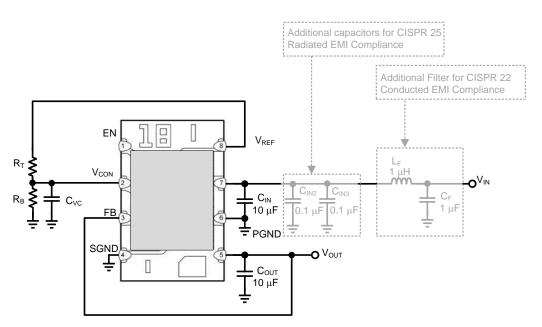
Figure 5. Evaluation Board Schematic
