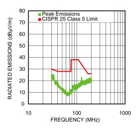
Figure 16. 30 MHz-200 MHz Horizontal 1A Load
