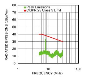
Figure 14. 5 MHz-30 MHz 1A Load
