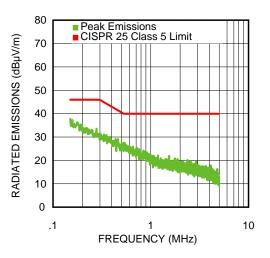
Figure 12. 0.15 MHz-5 MHz 1A Load
