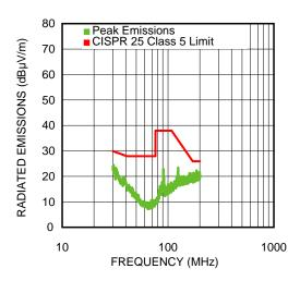
Figure 19. 30 MHz-200 MHz Vertical 650 mA Load
