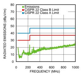
Figure 6. Radiated EMI 1A Load
