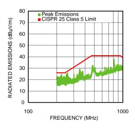
Figure 22. 200 MHz-1000 MHz Vertical 1A Load
