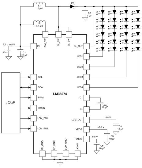
Figure 5. LM36274 Typical Schematic
