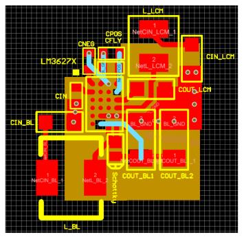
Figure 8. LM36274 PCB Layout
