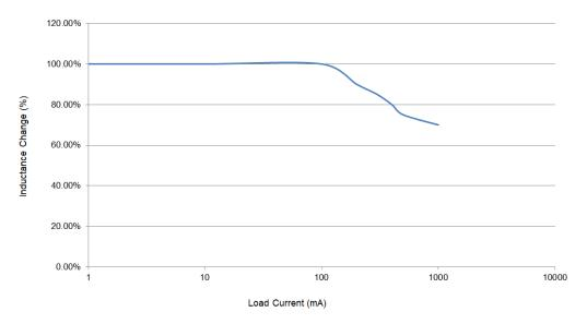
Figure 7. Inductance vs Load Current
