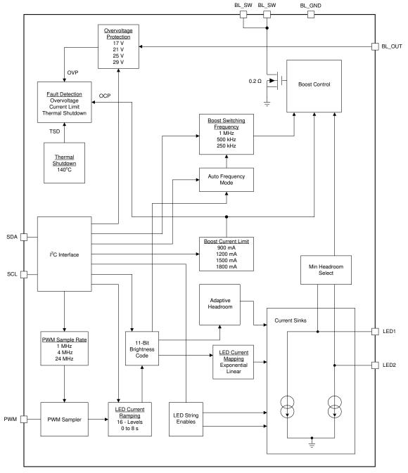
Figure 1. LM36273 LED Backlight Driver Unit
