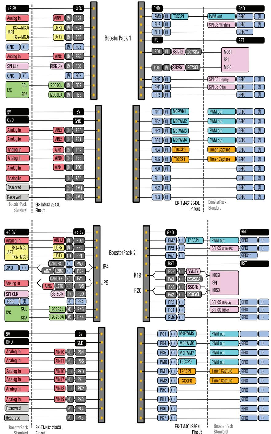
(I) indicates a GPIO pin that is interrupt capable.
