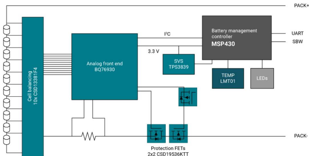
**Figure 1. Block Diagram of a Li-ion Battery Pack**
